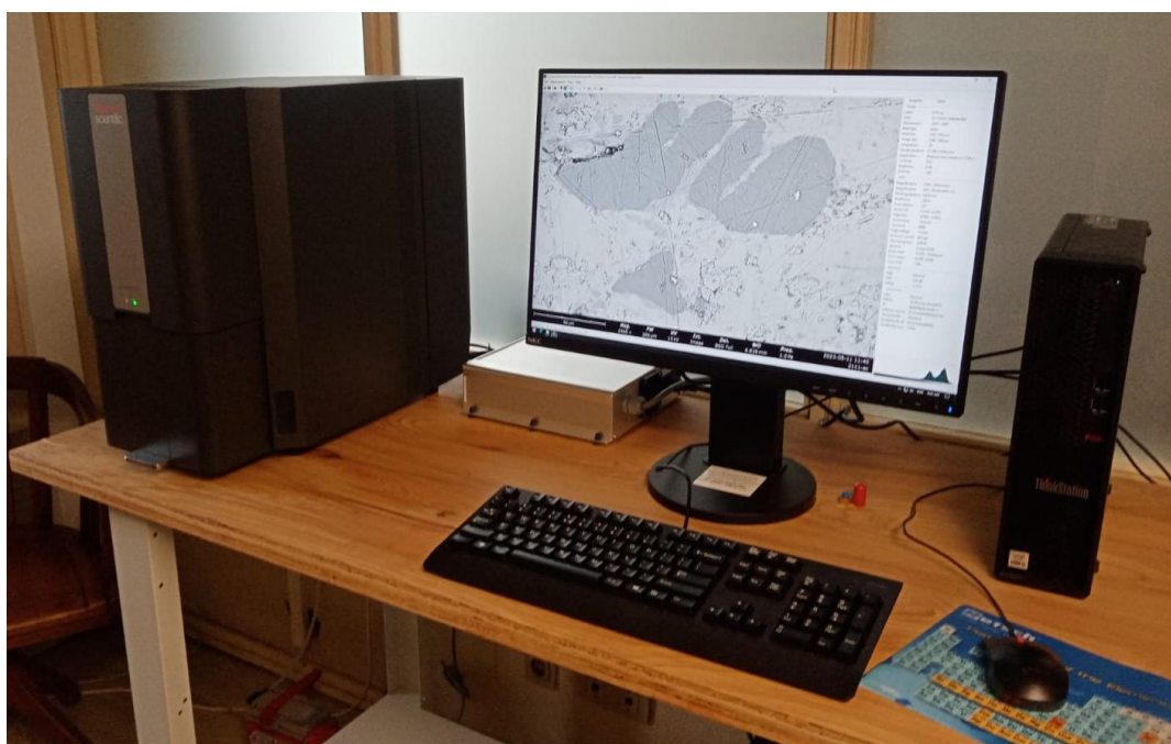
Fig. 24 Thermo Scientific Phenom ProX generation 6 desktop SEM with integrated EDS system.
