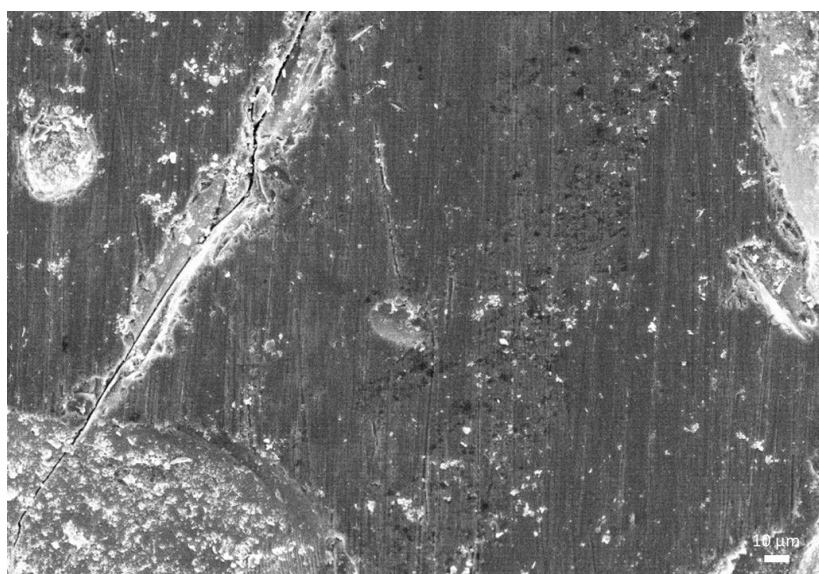
Fig. 35 SEM (BSE) micrograph of the Cu 12 Sb 4 S 11.5 Se as-cast sample
