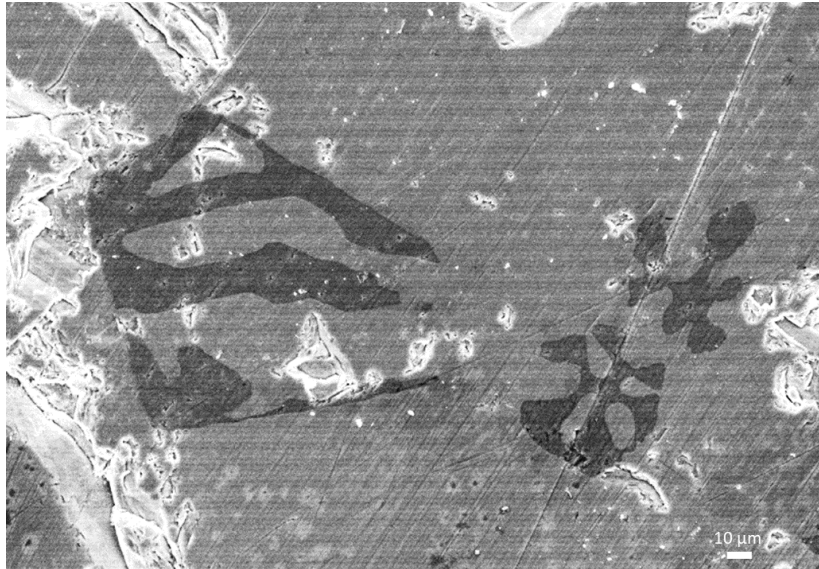
Fig. 126 Microstructures and pores observed in SEM imaging of the \text{Cu}_{11.5}\text{Ni}_{0.5}\text{Sb}_4\text{S}_{12}\text{Se} as-cast sample with 500x magnification. The dark phases are composed of nickel sulphides ( \text{Ni}_x\text{S}_y ). The lighter-shade phase is another tetrahedrite phase richer in sulphur than the matrix-tetrahedrite.
