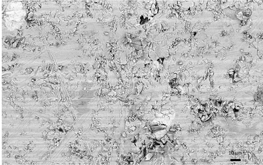
Fig. 159 Microstructures and pores observed in SEM imaging of the \text{Cu}_{10.5}\text{Ni}_{1.5}\text{Sb}_4\text{S}_{12.5}\text{Se}_{0.5} hot-pressed sample with 500x magnification. The dark phases are composed of nickel sulphides ( \text{Ni}_x\text{S}_y ). The light phases are composed of ullmannite ( \text{NiSbS} ).
