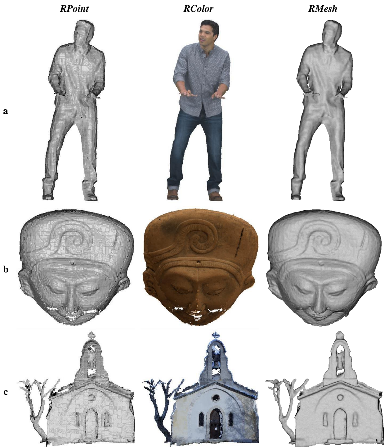
Figure 5.4: V-PCC coding artefacts: a) Loot ; b) Egyptian Mask ; and c) House without a Roof , when rendering with RPoint , RColor and RMesh .
