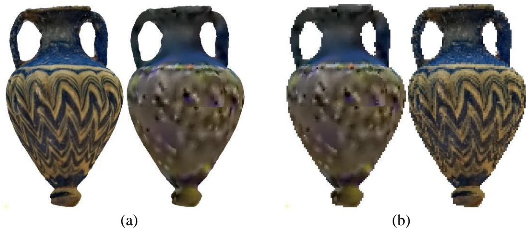
Figure 9.3: Amphoriskos decoded with G-PCC in octree mode and lifting color mode in the lowest rate; a) point clouds obtained for reference geometry with the reference (left) and decoded color, after recoloring (right), b) point clouds obtained for decoded geometry with the decoded color (left) and reference color, after recoloring (right).
