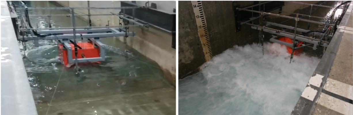
(a) Photograph of unbroken- (left) and broken-waves (right) induced by the horizontal displacement of the piston wave-maker and different initial free-surface elevations, respectively of 2.00 m and 1.85 m.
