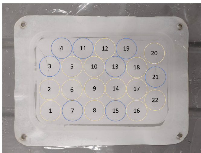
Figure 5.8: Membrane section from the SEPA unit with the twenty-two individual membranes marked. The circular membranes in yellow were utilized in the subsequent CNF testing.
