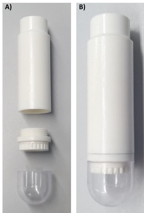
Figure 3.7: A) Disassembled components of the CNF device: cylindrical body, screw-on lid, and permeate chamber. B) Fully assembled CNF device, showing how the individual components integrate.
