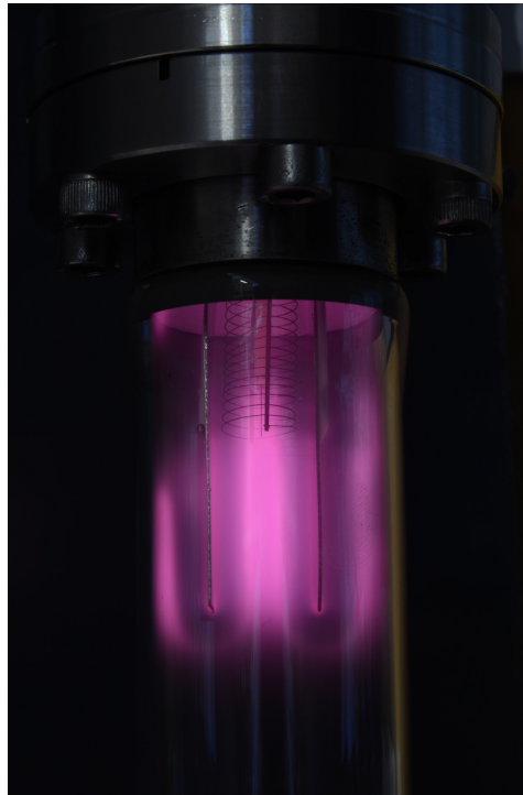
Figure 3.4.: Glow Discharge in the Chamber
