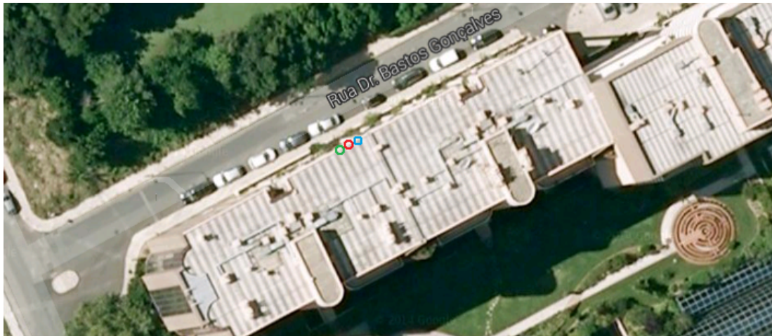
Figure 4.7: Position Results of Aquisition 1 - Real Position (Green) vs GPS Position (Blue) vs EGNOS Position (Red).
