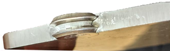
Figure 36 – Rivets attached to the top sheet after rupture of the bottom sheet in double riveted connection.
