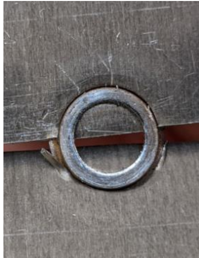
Figure 26 - Close-up view of the teared material from the joint under three-point bending flexural testing, in the DO orientation.
