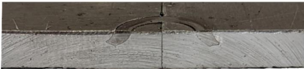
Figure 1 – Section view of a butt joint between two aluminium sheets using T-SPR technology.
