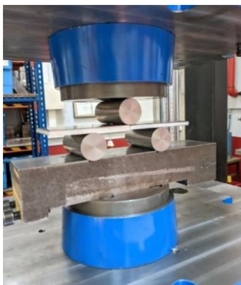
Figure 15 - Close-up view of the flexural tests' setup.
