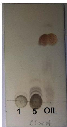
Figure 10.16 TLCs of samples from microcolumn and Oil as standard (TLC eluent: Chloroform)
