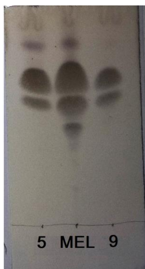
Figure 10.18 TLCs of samples from microcolumn and MELs sample (TLC eluent: Chlor/MeOH/H 2 O)
