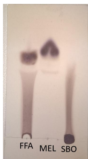
Figure 8.3 TLC with methanol as eluent. FFA - partially hydrolysed oil with free fatty acids
