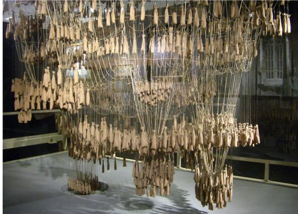
Figure 2.2: The hanging model of Colonia Güell
