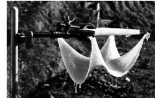
(a) Resultant shape for pinned corners and fibers parallel to the edge, adapted from [16]
