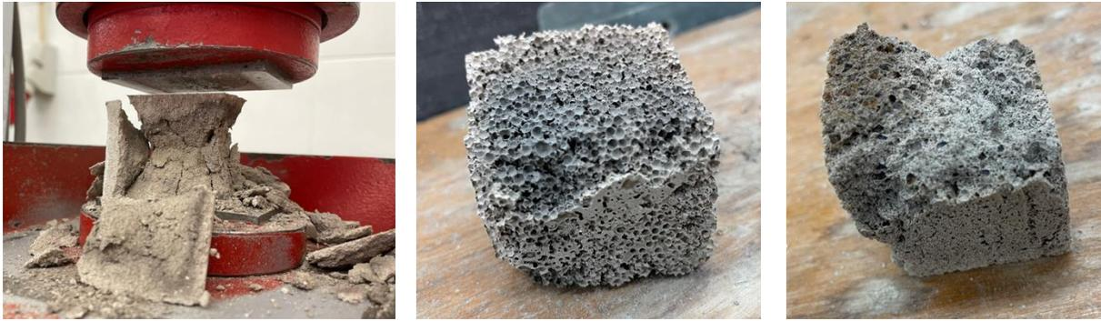
Figure 17. Specimens after residual compressive strength test: Lime.m (left), EPS.m (middle), Aero.m (right)
