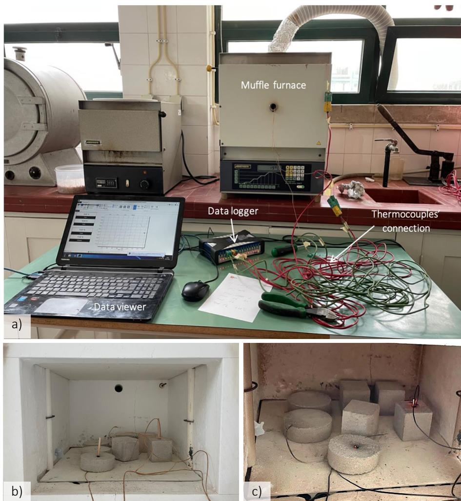
Figure 12. Test setup: a) general view; Specimens' placement post heating b) Lime.m and c) EPS.m and Aero.m
