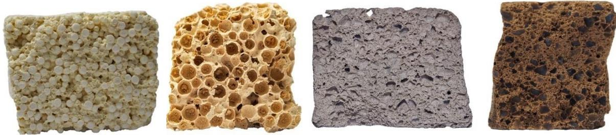
*Figure 23. Zoomed photos. From left to right: initial EPS.m, post-heating EPS.m, initial Aero.m, post-heating Aero.m*
