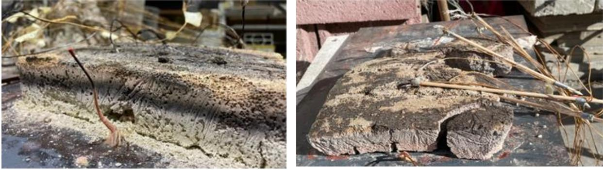
Figure 28. Thermal mortars post testing: EPS.m (left), Aero.m (right)
