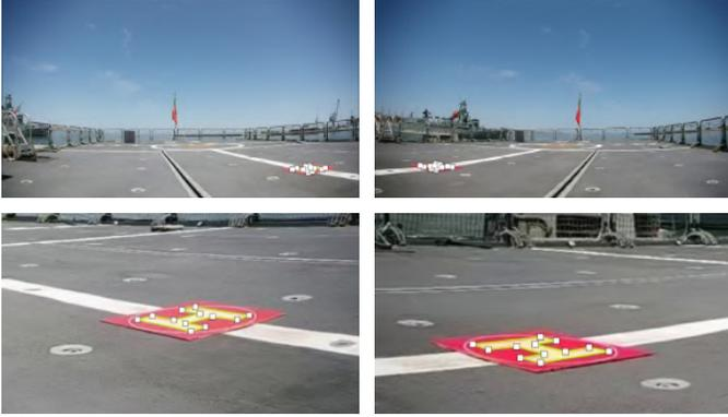
Fig. 7. Images used for camera calibration (*top*) and marker detail and annotations (*bottom*).
