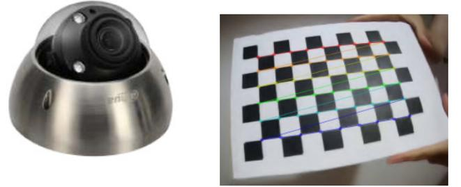
Fig. 5. *Dahua* camera (left) and chessboard calibration pattern (right).
