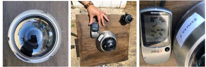
Fig. 21. Dahua camera (*left*), wooden support designed to perform data acquisition (*center*) and GPS (*right*).
