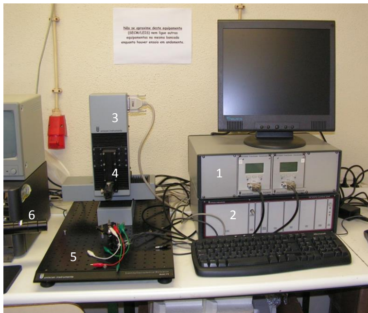
Figure 2.21. Picture of Uniscan M370 Electrochemical Workstation: (1) bi-potentiostat PG580R, (2) electronic rack (electronics control unit), (3) xyz scanning head, (4) original tip holder, (5) optical table with anti-vibration system and (6) video microscope.
