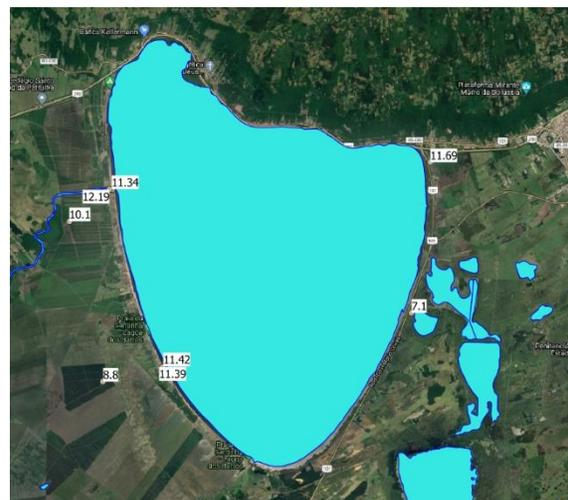
**Figure 51 Groundwater Level recorded in wells around the lake in m.a.s.l. at 23/10/2014.**
