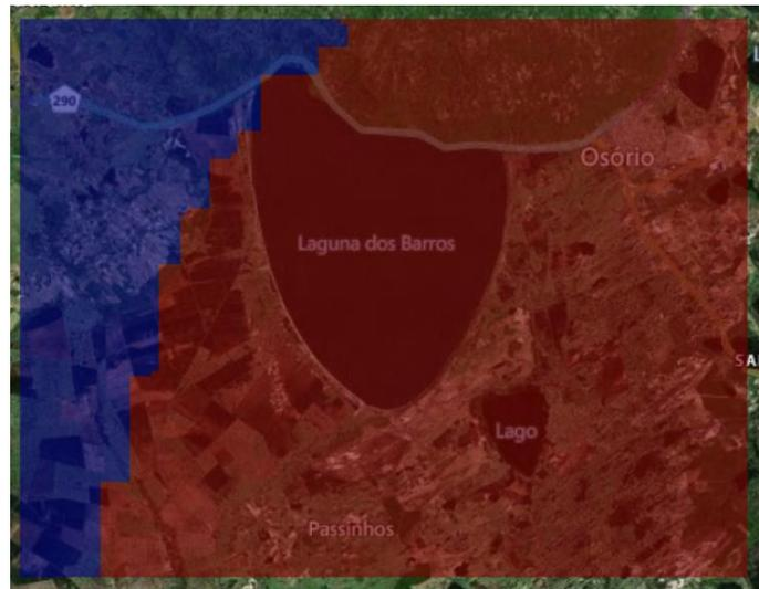
**Figure 44 Sub and Top Soil distribution in the area, in Blue the Planossolos and in Red the Arenossolos (FAO/IIASA/ISRIC/ISS-CAS/JRC, 2009)**
