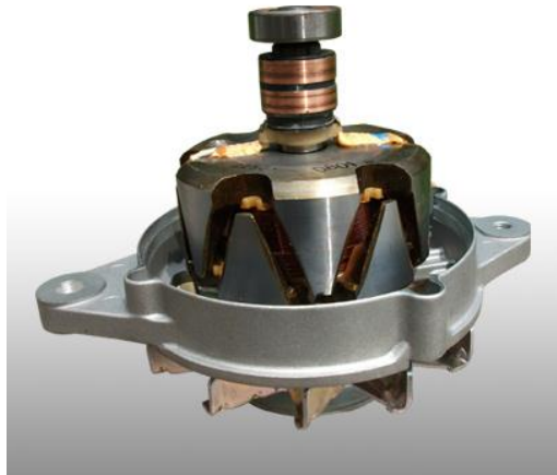
FIGURE 3.5 – Representation of the Rotor of a Lundell or Claw-Pole Alternator
