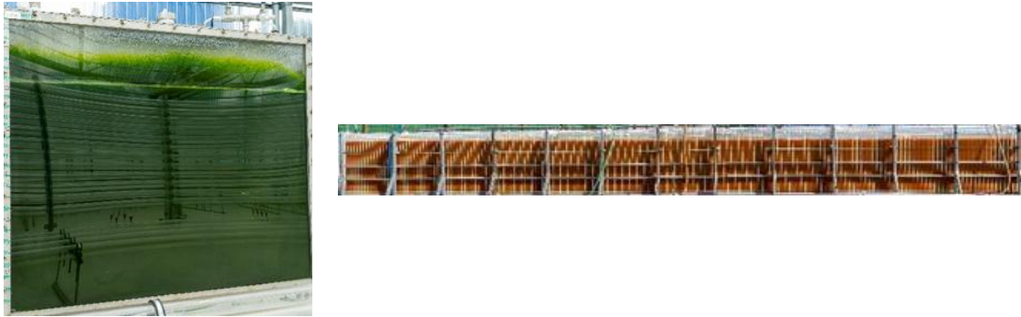
Figure 1: Glass (left) and plastic (right) flat panel photobioreactors. Courtesy of A4F.
