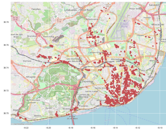
Figure 4-15 - Properties with higher vulnerability to earthquakes, based only on soil type (VULSismo>=3)
