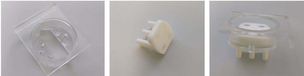
Figure 3.8: Photographs of the PMMA holder (**left picture**) and of the Teflon spacer (**center picture**). By positioning the spacer in the holder and placing it on the well with agarose, the spacer shapes the casting mould according to desired specifications.
