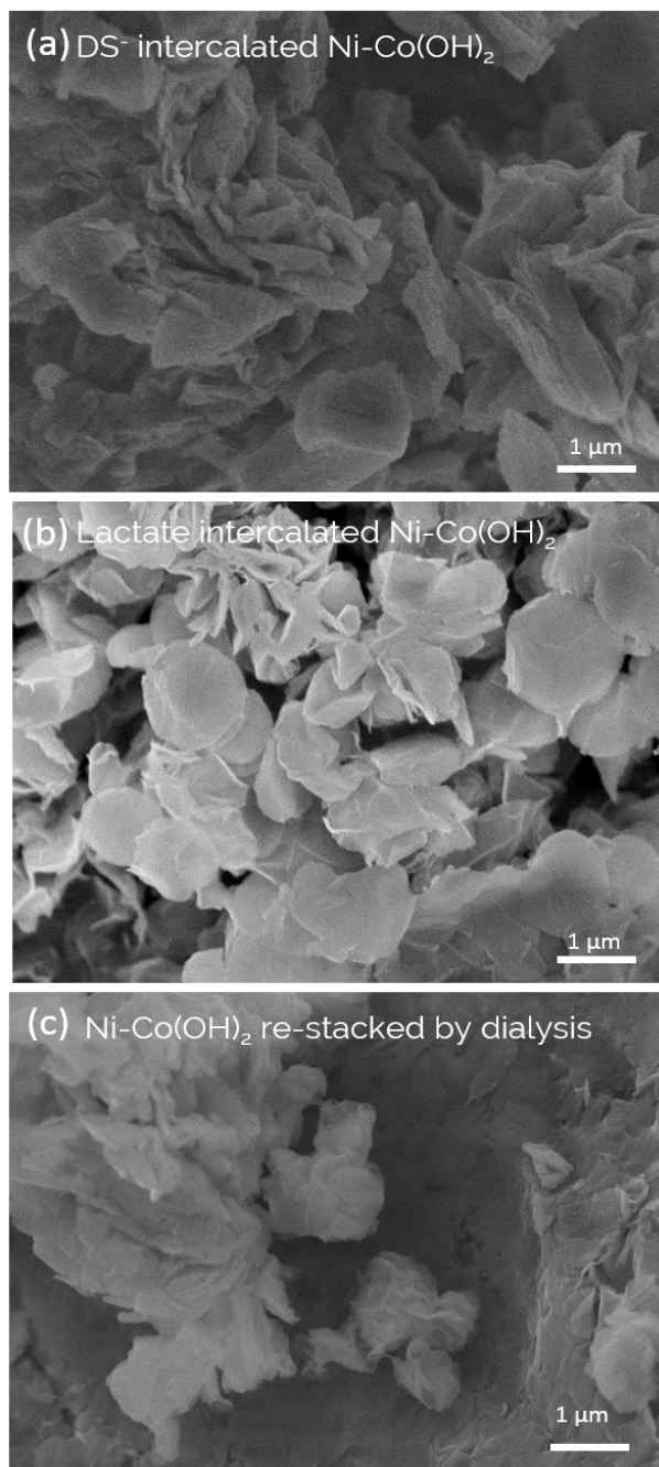
Fig. 3.5.4 Scanning Electron Microscopy images of (a) DS-NCOH, (b) Lac-NCOH and (c) restacked nickel-cobalt hydroxide nanoslabs by dialysis after exfoliation in distilled water (NCOH-DIAL).
