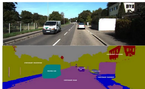
Figure 1.3: Example of the result of segmentation on a typical road scenario.
