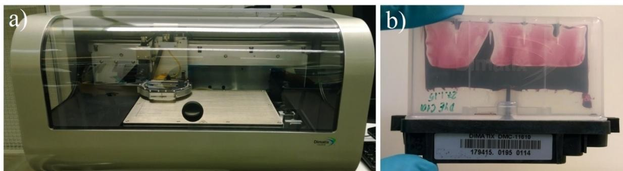
**Figure S4.** The inkjet-printer used in this study. a) Fuji Film's Dimatix Material Printer, Model DMP-2800, and b) printer cartridge filled with dye C101 solution.
