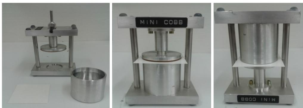
**Figure 10:** Cobb test setup and procedure steps: **a)**  $7 \times 7 \text{ cm}^2$  FBS and Mini Cobb with its water container ring filled with DI, **b)** FBS is fastened between the security plate and water container and **c)** FBS is exposed to water for 24 h in Mini Cobb setup in the inverted position
