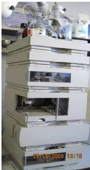
Figure 27 – HPLC used in laboratory.
