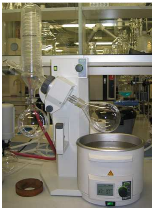
Figure 22 – Rotary evaporator used to eliminate the water.
