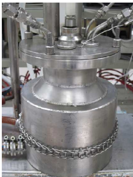
Figure 20 – Autoclave reactor of 1l.
