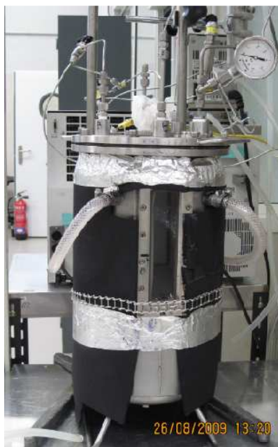
Figure 21 – Autoclave reactor of 8l.
