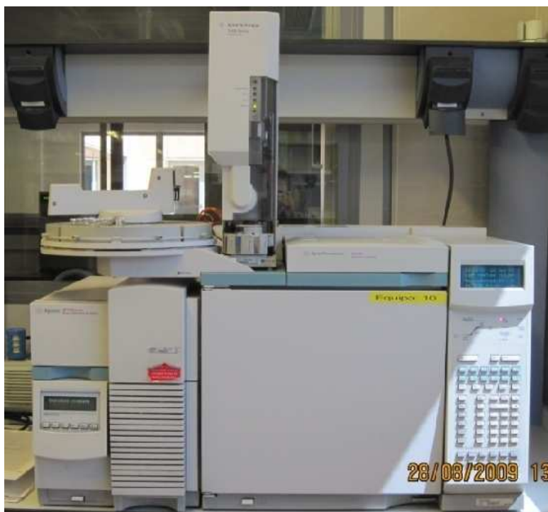
Figure 28 – Gas chromatograph - mass spectrometer used in laboratory.
