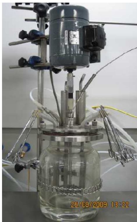
Figure 16 – Glass reactor of 1l with the motor that promotes the agitation.
