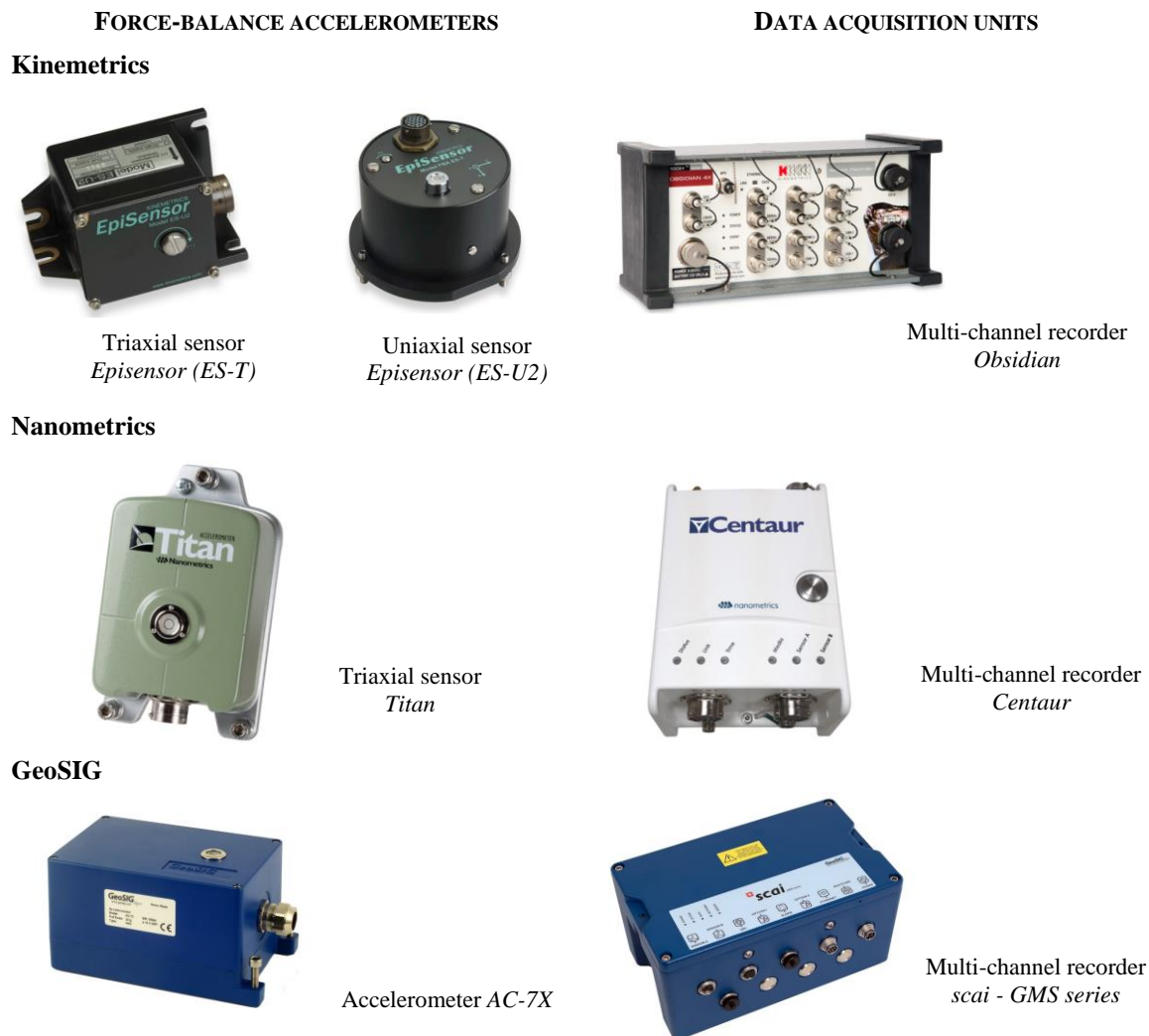
Fig. 4.5 Examples of available equipment for SSHM systems. Accelerometers and data acquisition units.
