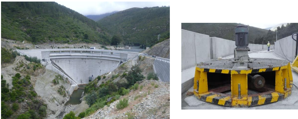
Fig. 2.20 Alto Ceira II arch dam (41 m high), Portugal. Eccentric mass shaker used in forced vibration test.
