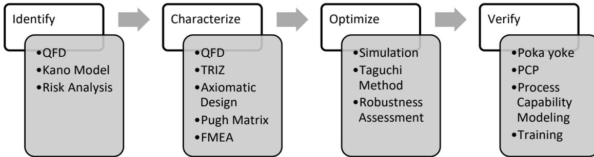
Figure 6 Phases and tools for engineering design process
