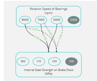
Appendix G Figure 3 Correlations Between "Rotation Speed of Bearings" and "Internal Steel Strength on Brake Discs"
