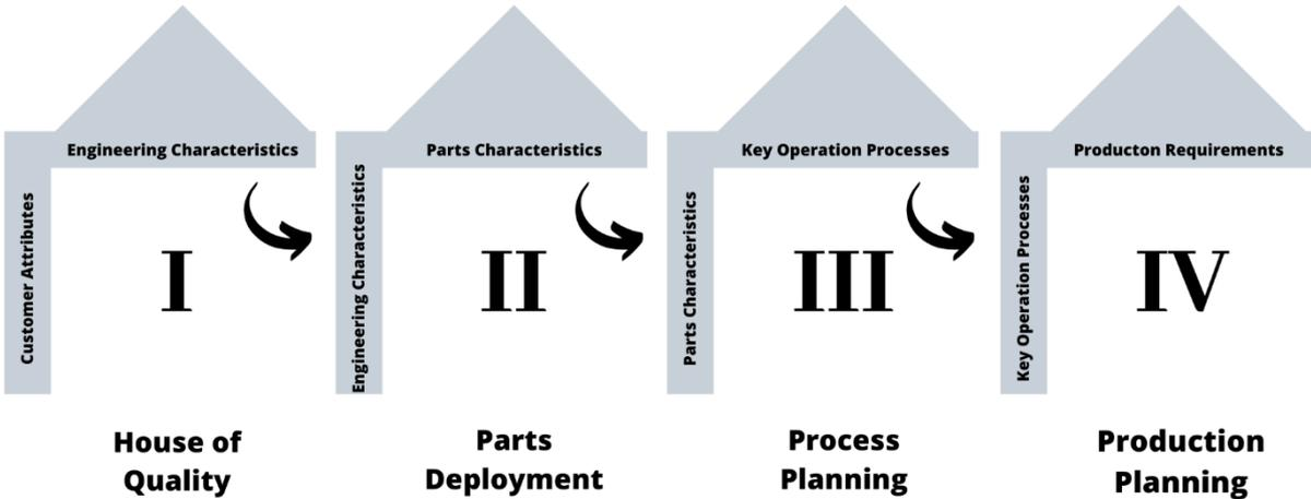
Figure 7 The four QFD houses adapted from Hauser and Clausing (1988)
