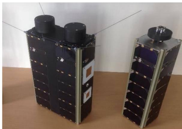
Figure 1.5: QUBE-II (left) and QUBE-I (right) [5]
