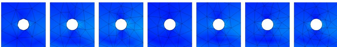
**Figure 5.10:** Mesh refinement around the middle hole in Rib-3 (from left to right)
