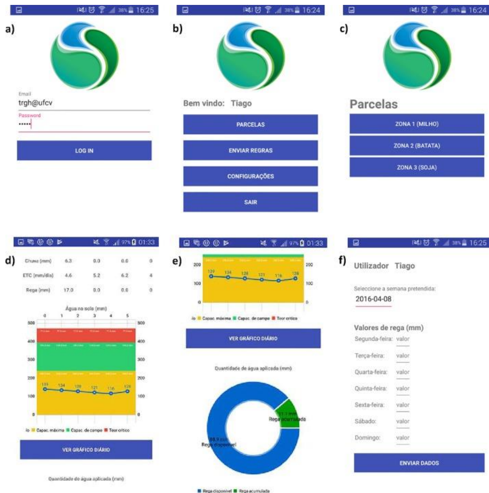
Figure 3.2-6 Smart phone application for accessing the IrrigaSys results. a) login menu; b) main menu; c) menu with registered plots; d) and e) menu with the weather forecast, evolution of soil water contents, and cumulative irrigation amounts; and f) menu for providing past irrigation events to feed the system.
