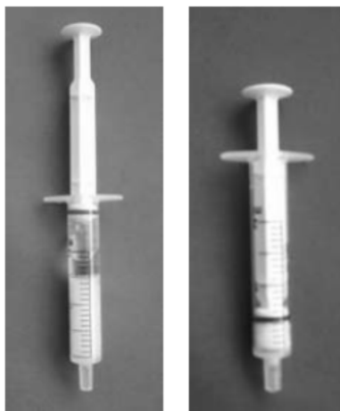
Cryogel BasicE: hydrated and compressed with a plunger plugs (right) inside a plastic column.
