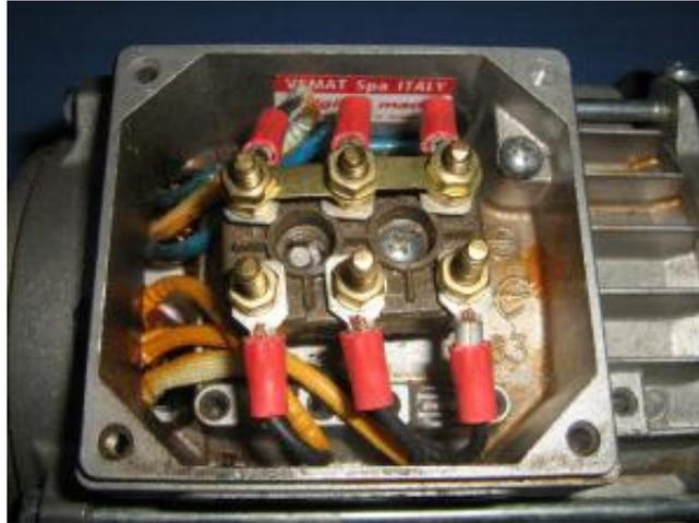
Figure 4.3: Example of an induction motor junction box showing a star windings connection - motor of the IST Energy Laboratory.
