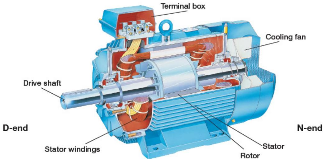
Figure 3.3: Three-phase, squirrel cage induction motor with a transversal cut [tesinasalvatorecopola.altervista.org, 2017].
