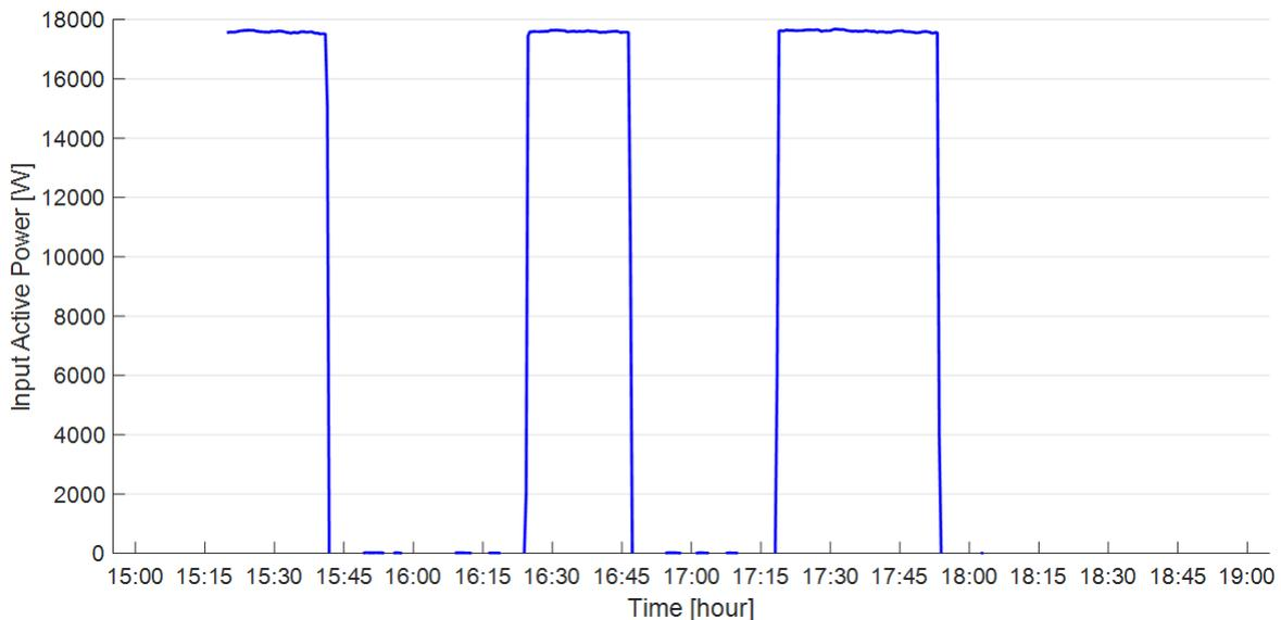
Figure 4.15: Example of an induction motor load profile, obtained from one of the motors analysed in this thesis (BPC1), located on the Cold Central of the IST Alameda Campus North Tower.
