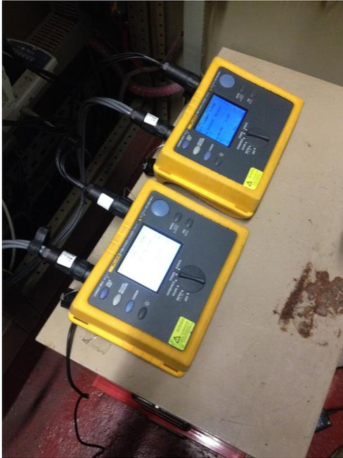
Figure 4.9: Two Flukes retrieving data over time - Cold Central of the IST Alameda Campus North Tower.
