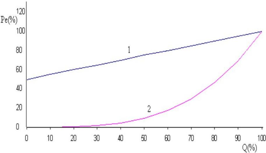
Figure 3.9: Electric Power vs. Flow for two flow control methods: 1 - Choking Valve; 2 - VSD [6].
