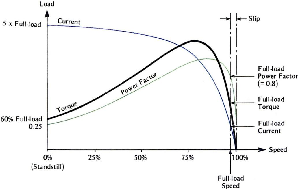
Figure 3.4: Typical torque-speed, current-speed and power factor-speed curves for an induction motor [emadrlc.blogspot.pt, 2017].
