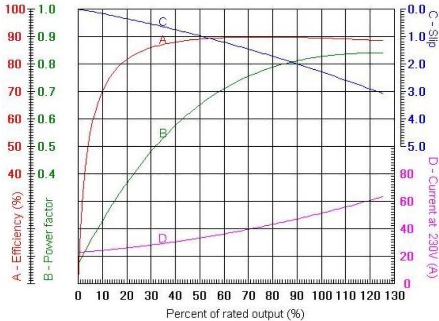
Figure 3.5: WEG W22 - Cast Iron Frame - Standard Efficiency, 15 kW curves [4].
