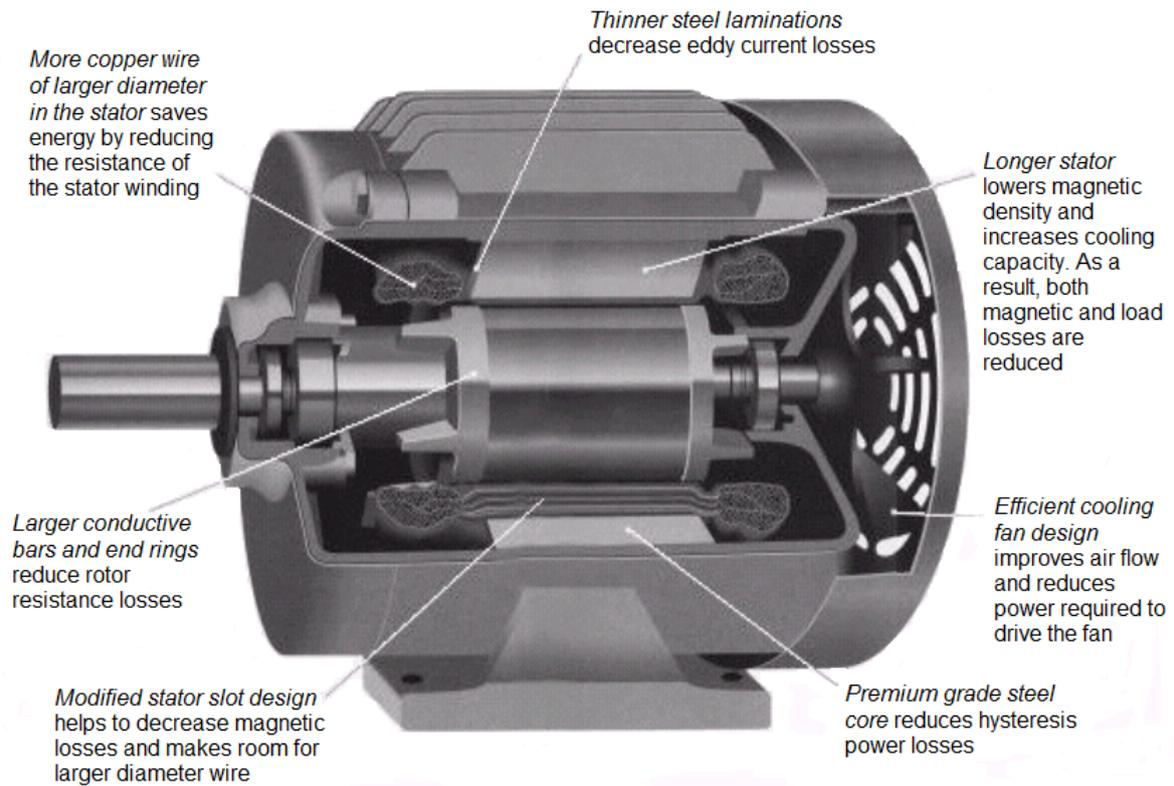
Figure 3.6: High-efficiency motor construction details [5].
