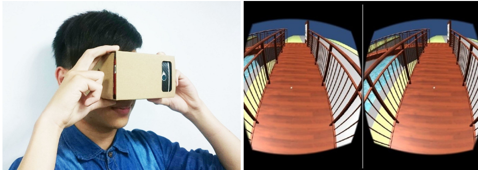
(a) A user visualizing the virtual representation of the FRP bridge through the use of the Google Cardboard Oculus (b) The FRP bridge inside the virtual environment
