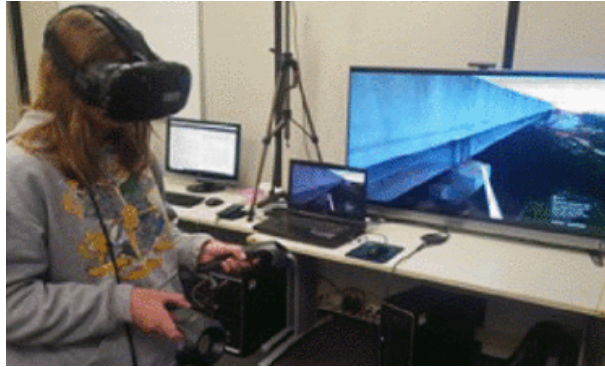
Figure 2.5: User performing a bridge inspection with ImSpector [Veronez et al., 2019]
