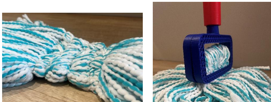
Figure 20. Complete assembly including the sewn fibers, the first 3D-printed piece, and the mop handle
