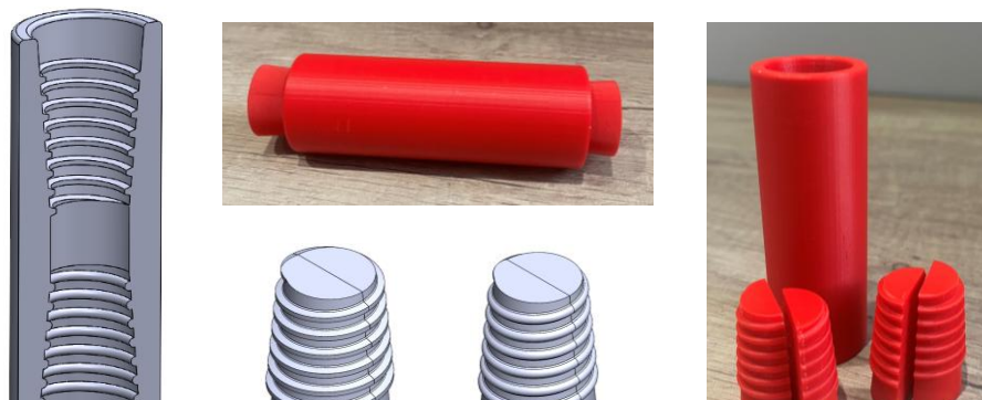
Figure 19. 3D-printed and CAD models of the mop handle with both thread types
