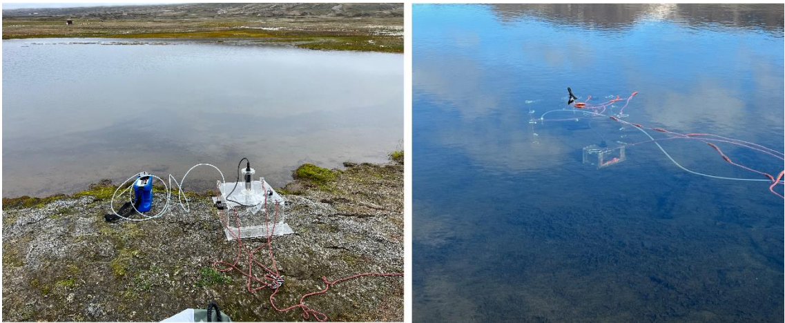
Figure VII.III.1. Photograph of the benthic flux chamber system in the margin of the lake (left) and during the experiment (right).
