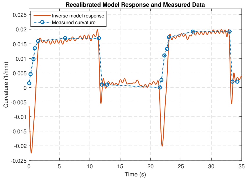
Figure 4.24: Calibrated inverse model response and measured actuator curvature.
