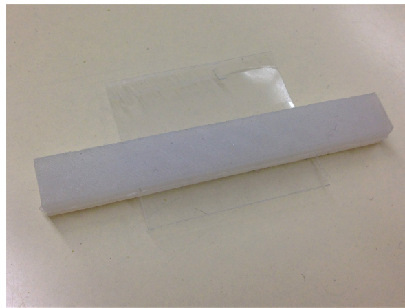
Figure 3.1: Two silicone parts being joined into a type 1 encapsulation. Note the plastic plate forming a slot for the IPMC.
