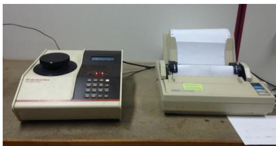
**Figura 3.11 - Picnómetro Micromeritics Accupyc 1330.**
