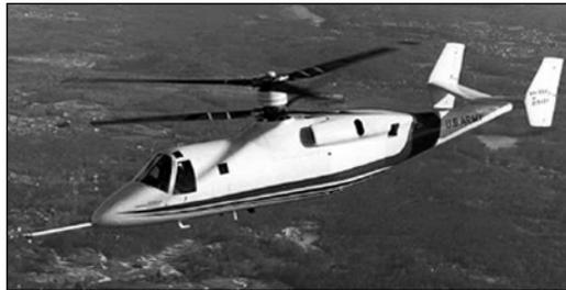
(a) XH-59A Advancing Blade Concept technology demonstrator helicopter without auxiliary propulsion.
