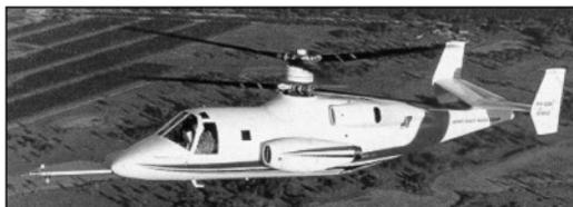
(b) Second version of the XH-59A compounded in thrust with two J60-P-3A turbojet engines.
