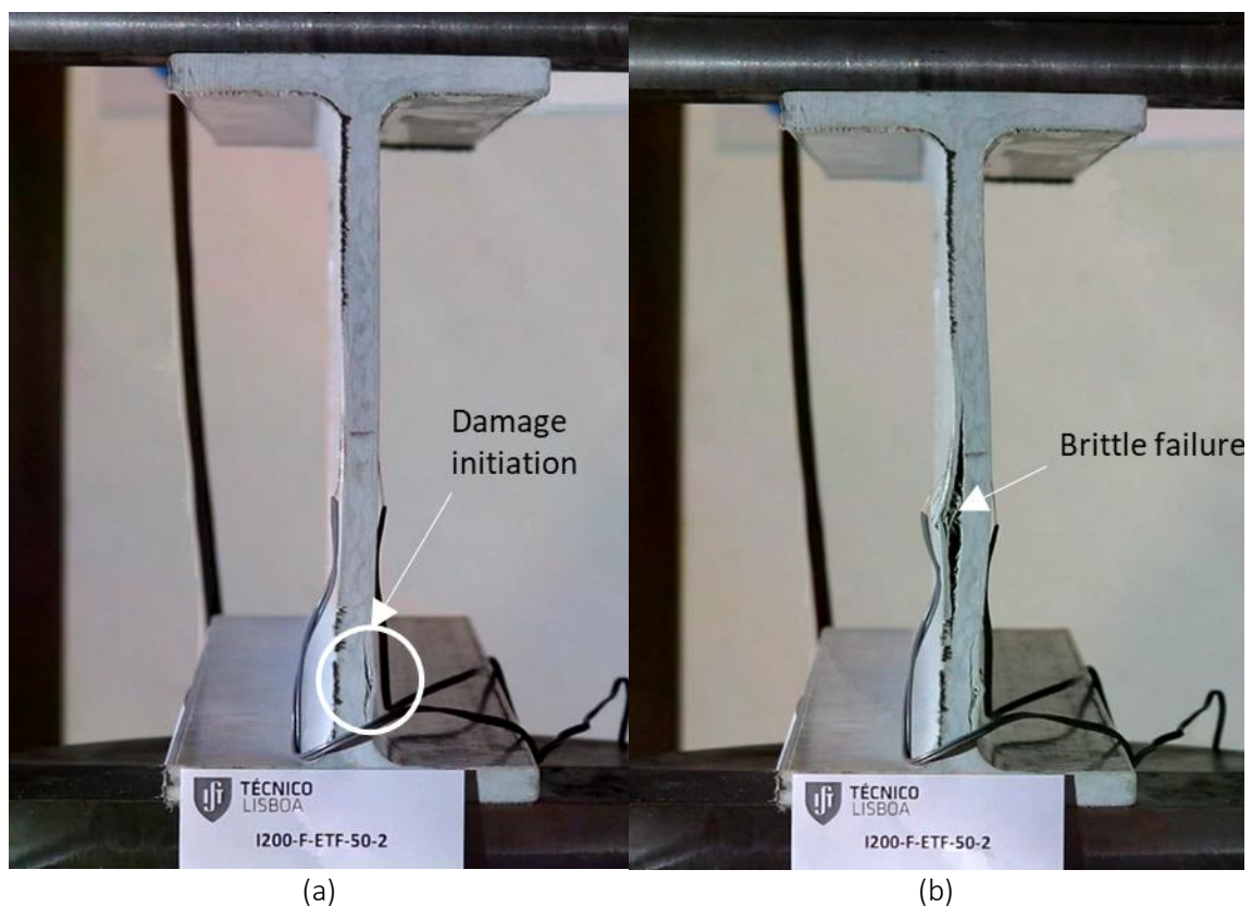
Figure 6.8: Failure mode of I200-F-ETF-50-2 specimen: (a) damage initiation near the bottom web-flange junction; followed by (b) brittle failure due to web-buckling.
