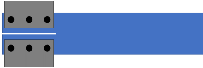
Figure 2.9: DCB test specimen geometry.
