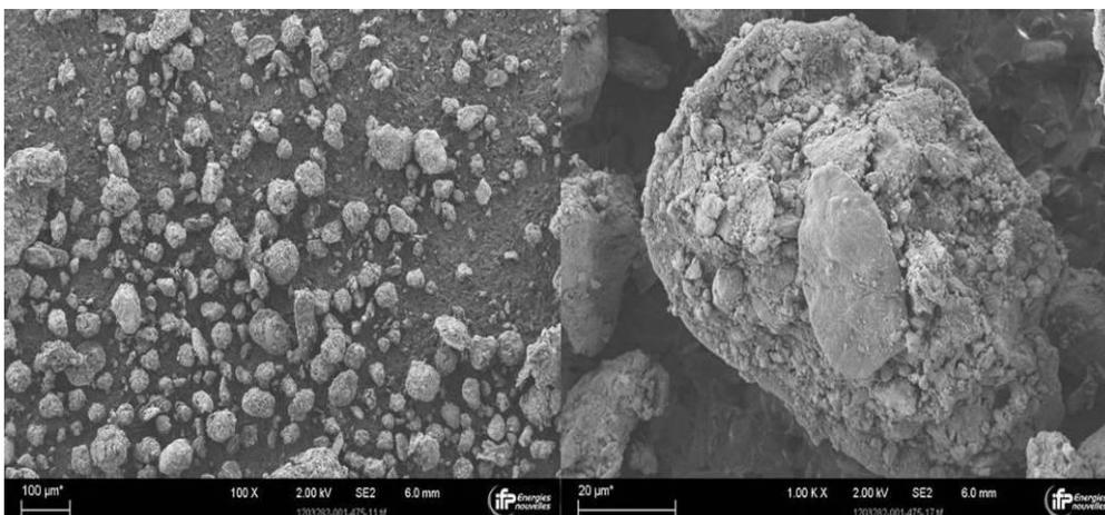
Figure 47 - SEM images of product 120615 (scale bar of 100 and 20  $\mu\text{m}$ )
