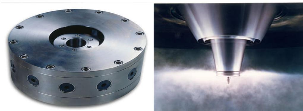
**Figure 8 - Rotary Atomizer [43], [44]**
