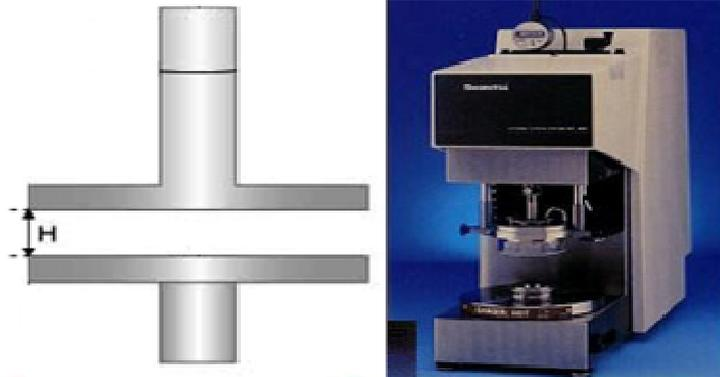
Figure 34 - Parallel plates configuration and rheometer used in this work
