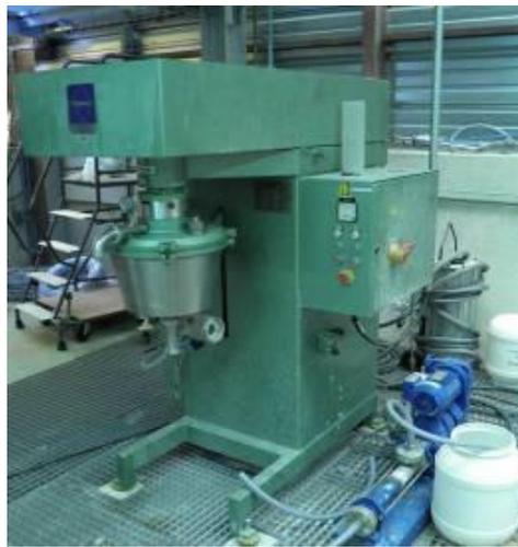
**Figure 23 - Ball Mill equipment used in this work**
