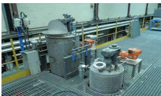
Figure 19 – Image of mixing vessels used for preparation of acid and basic solutions
