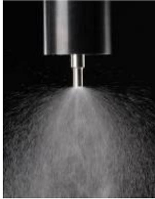
Figure 11 - Ultrasonic nozzle [49]
