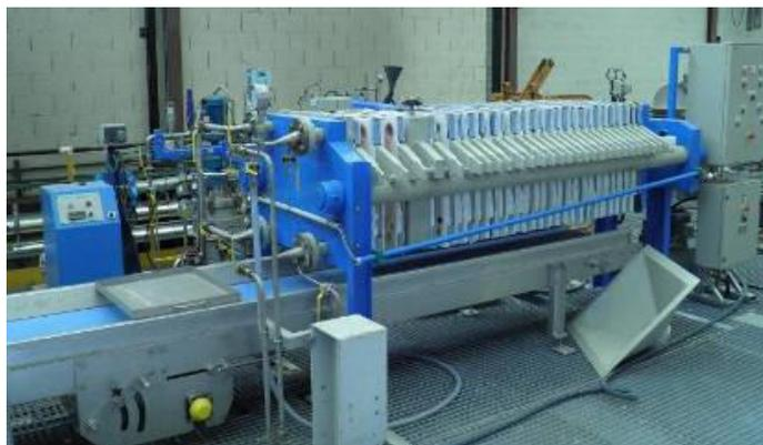
Figure 21 – Picture of the industrial Filter Press used in this work
