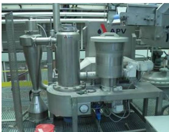
Figure 22 – Picture of the Spin Flash dryer equipment used in this work
