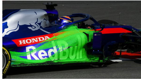
(b) Flow-vis paint. From [24].
