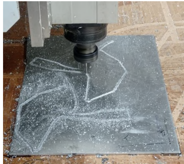
(b) Aluminium rear wing supports.
