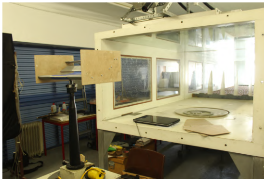
(a) Rear wing testing.
