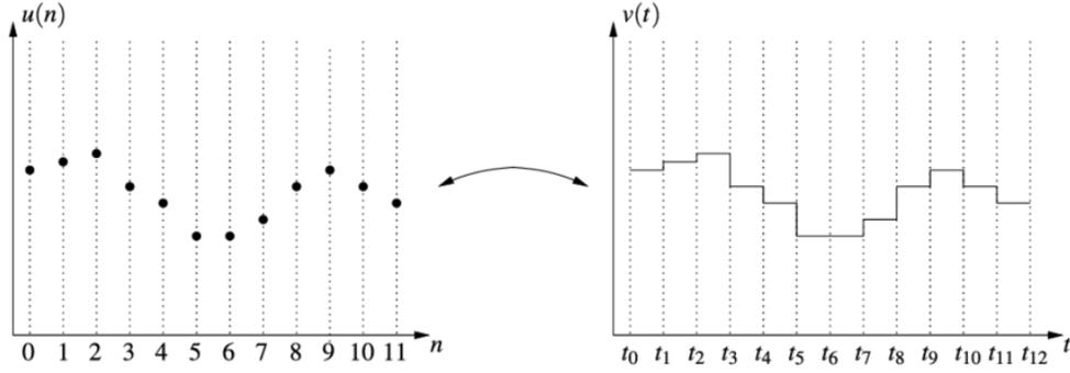
Figure 3.3: Zero order hold input scheme illustration [62].
