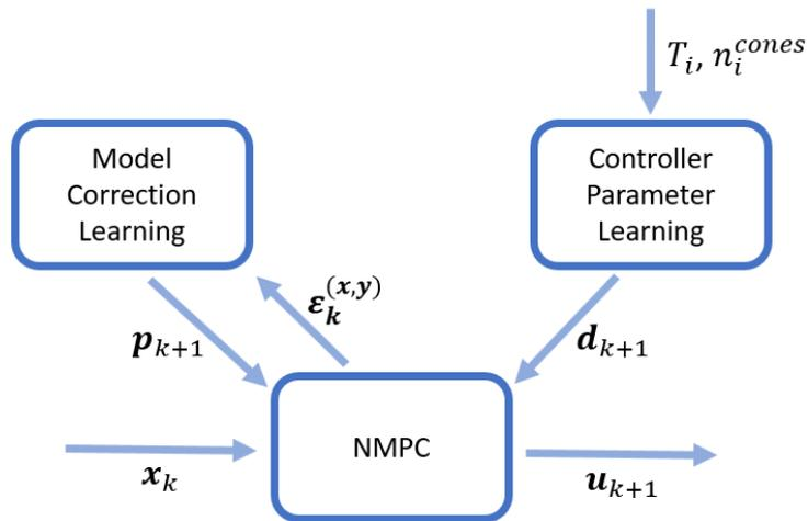
Figure 6.2: ROS nodes for the developed control architecture.
