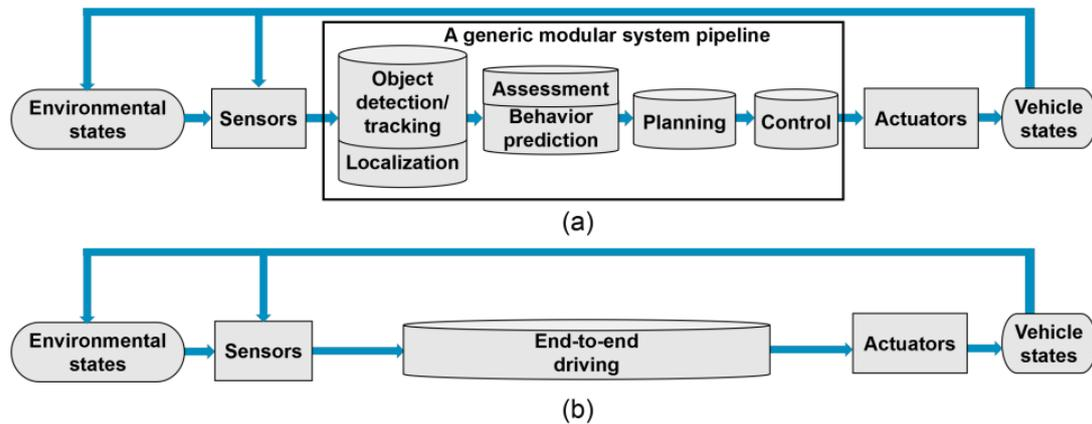
Figure 1.3: Typical autonomous driving pipeline: (a) a generic modular system, and (b) an end-to-end driving system [8].
