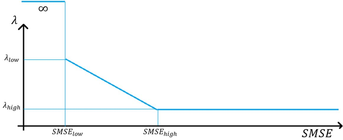
Figure 3.7: Schedule template function of the damping parameter,  $\lambda$ .
