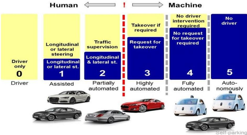
Figure 1.1: Levels of autonomous driving according to SAE J3016 [1].
