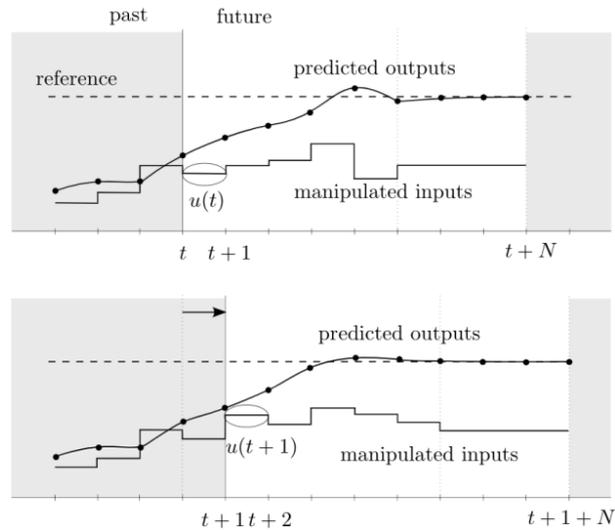
Figure 2.1: Receding Horizon principle [47].
