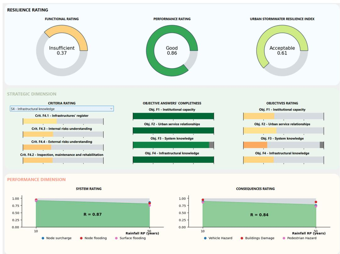
Figure 5-10. RESILISTORM-tool: example of the Resilience Dashboard for testing a stormwater service
