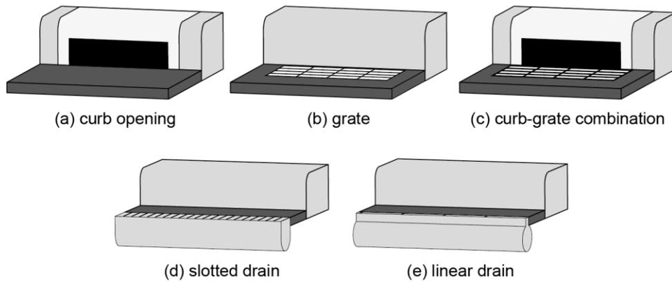
**Figure 3-1.** Conventional types of stormwater inlet devices
