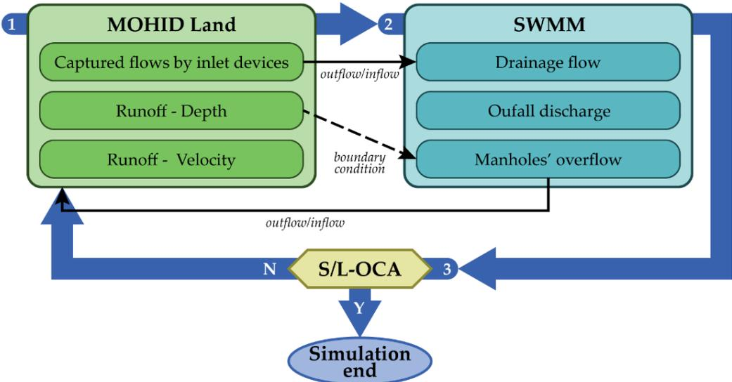
Figure 4-5. SWMM/Land coupling steps and simulation cycles
