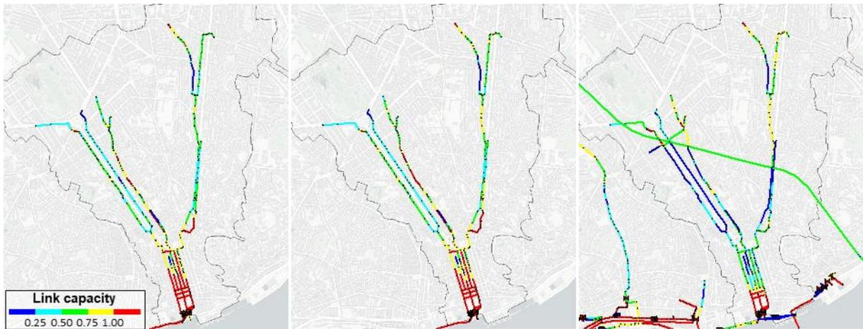
**Figure 6-26.** Minor system sewer capacity at the critical event time for the 100-year return period rainfall at CS (left), BAU (center), and FS (right) in the Historic Downtown catchment
