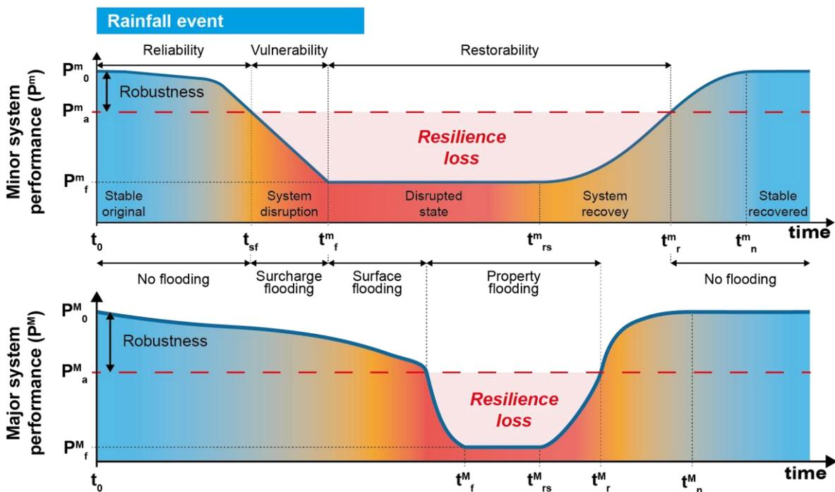
Figure 3-15. Theoretical system performance curve applied to stormwater systems (Mugume et al., 2014; Hosseini et al., 2016; Matzinger et al., 2019)
