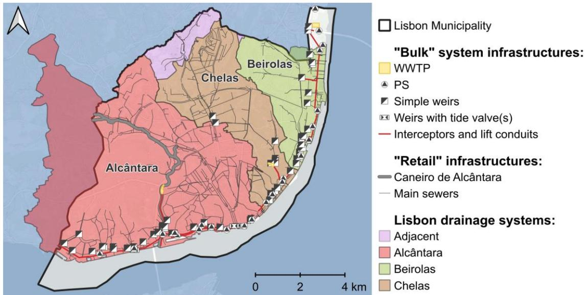
Figure 6-8. Lisbon drainage systems and main infrastructure
