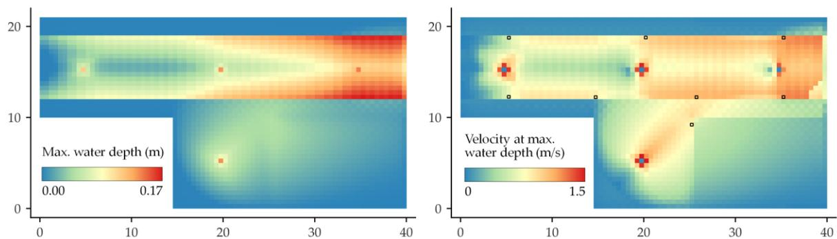
**Figure 4-9.** Synthetic case study: resulting maximum water depth (left) and velocity modulus at maximum water depth (right)
