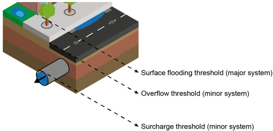
**Figure 3-7.** Stormwater flooding thresholds (adapted from Butler et al., 2018)
