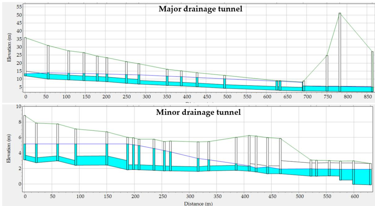
**Figure 4-17.** Albufeira case study: hydraulic profile at maximum water depth of the major and minor drainage tunnels for the 10-year return period rainfall (top and bottom, respectively)
