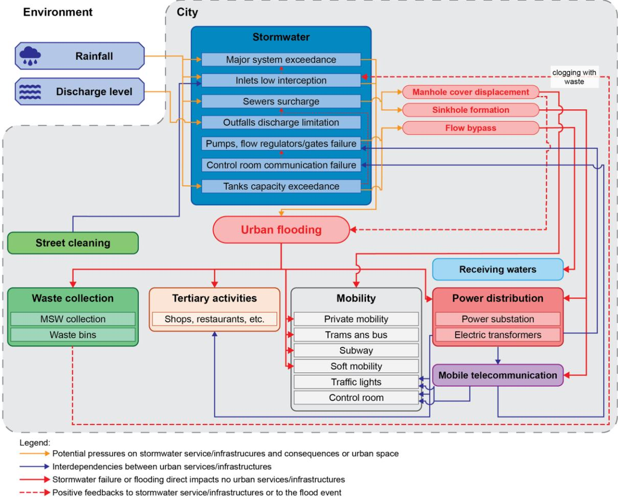
Figure 3-13. Potential cascade effects due to stormwater failure and flooding direct impacts
