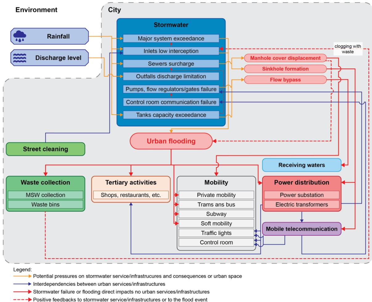
Figure 5-2. Generic cascade chain and feedback for urban stormwater system failure
