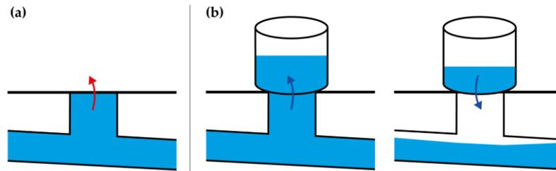
**Figure 4-1.** Graphical representation of 1D models dealing with manhole overflow: (a) lost from the system or (b) ponded in virtual storage volume
