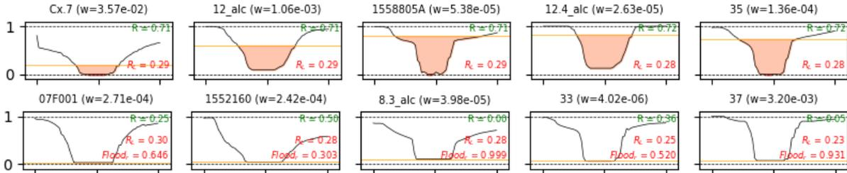
**Figure 6-34.** Examples of node surcharge (top) and flooding (bottom) performance curves obtained for the CS-2020 Situation in the Alcântara catchment. The x-axis represents the duration of the event under analysis (5 hours), and the y-axis represents the performance relative to the corresponding state variable. The w value stands for the node weight.
