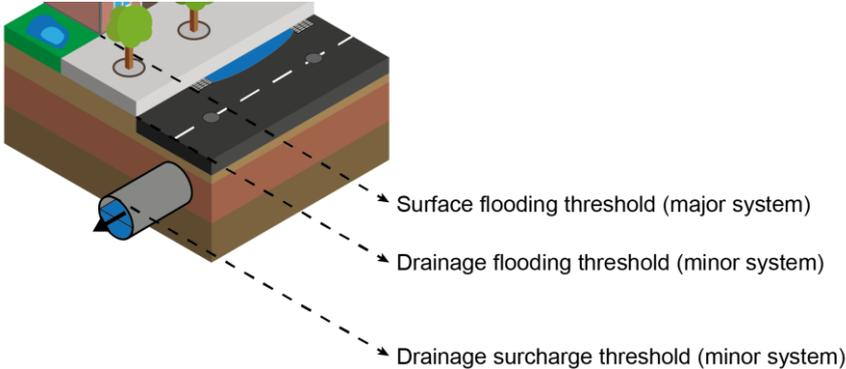
**Figure 5-1.** Stormwater flooding design thresholds
