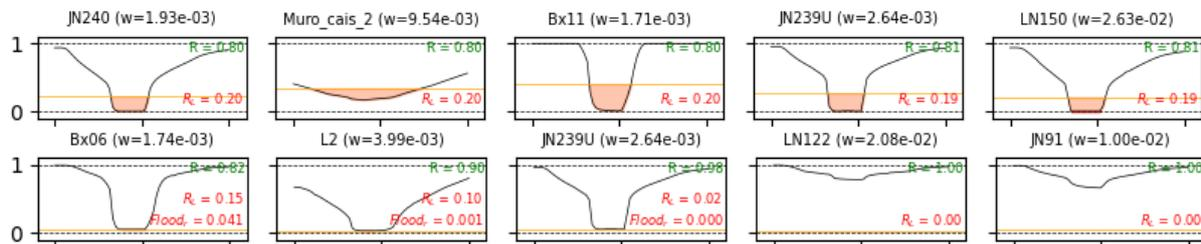
**Figure 6-24.** Examples of node surcharge (top) and flooding (bottom) performance curves obtained for the 100-year return period rainfall in the Current Situation of the Historic Downtown catchment. The x-axis represents the duration of the event under analysis (5 hours), and the y-axis represents the performance relative to the corresponding state variable. The  $w$  value stands for the node weight.
