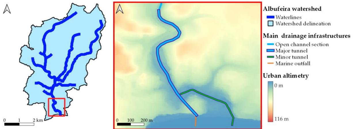
**Figure 4-10.** Albufeira watershed and main urban drainage infrastructures and altimetry.
