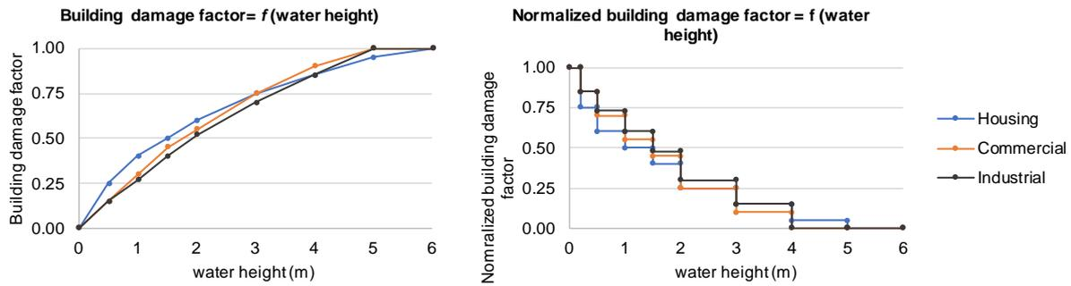
**Figure 6-4.** Curves of damage factor and normalized damage factor to buildings
