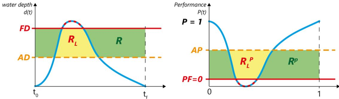
Figure 5-6. State variable performance (left) and normalized performance curve (right)
