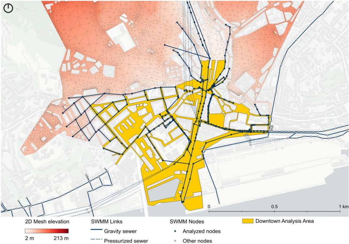
**Figure 6-32.** Critical area and drainage nodes considered for the Alcântara catchment Performance Dimension assessment
