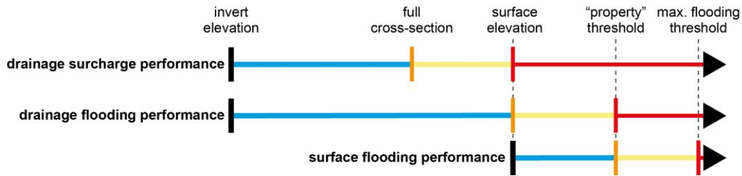
**Figure 5-7.** Reference and threshold values of stormwater performance curves
