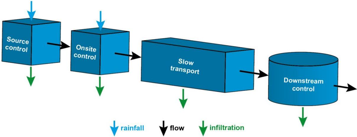
**Figure 3-5.** Categories and main fluxes of water in sustainable urban drainage facilities (adapted from Stahre, 2008)
