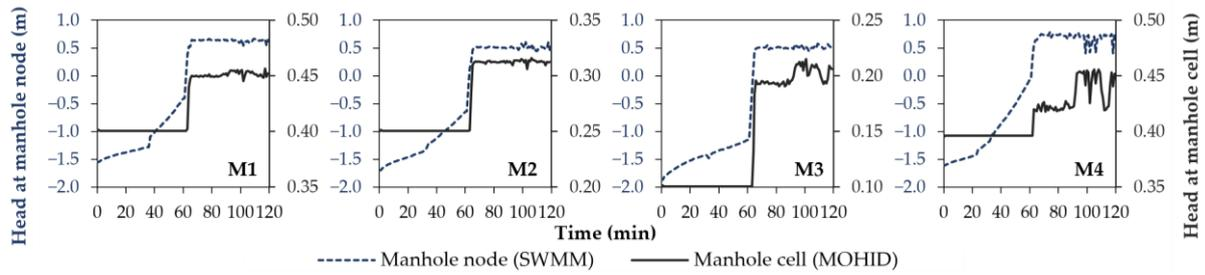
**Figure 4-8.** Synthetic case study: resulting water head at manholes (SWMM nodes) and at respective 2D cell (MOHID)
