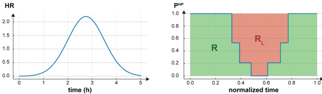
**Figure 6-3.** Example of a flood hazard for pedestrians' curve (left) and normalization into the respective performance curve (right)
