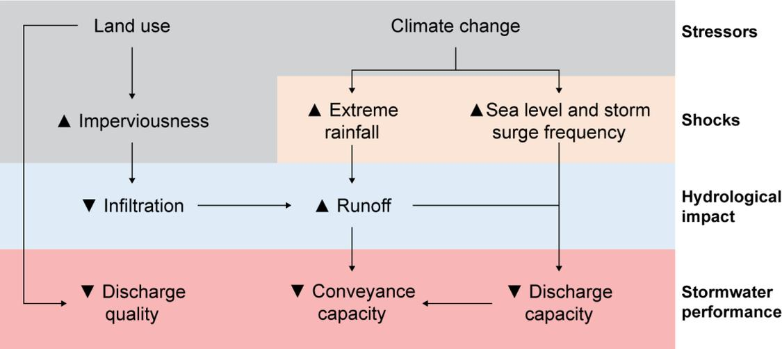
Figure 3-10. Flowchart of stormwater’ stressors and shocks and their impact on stormwater performance
