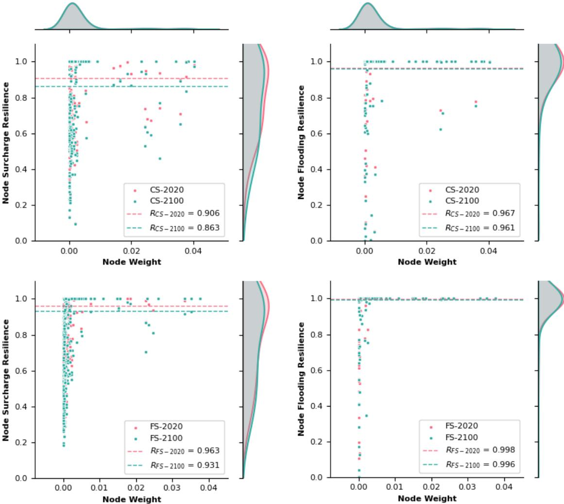
**Figure 6-33.** Plots of node weights vs. node surcharge resilience (left) and node weights vs. node flooding resilience (right) for the Current Situation (CS) and Future Situation (FS) in the Alcântara catchment
