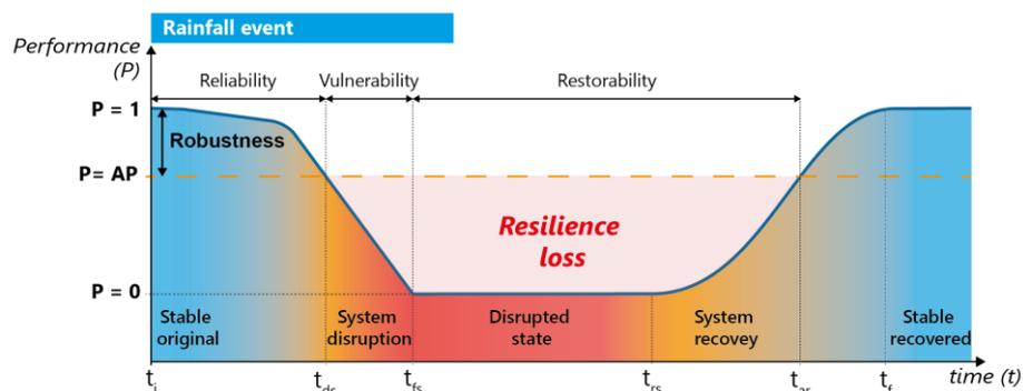
**Figure 5-5.** Theoretical generalized performance curve for stormwater systems
