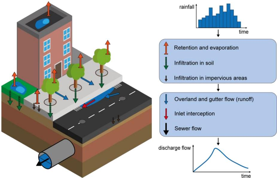
**Figure 3-6.** Processes from rainfall to runoff and discharge flow (adapted from Loucks and van Beek, 2017; Rammal and Berthier, 2020)
