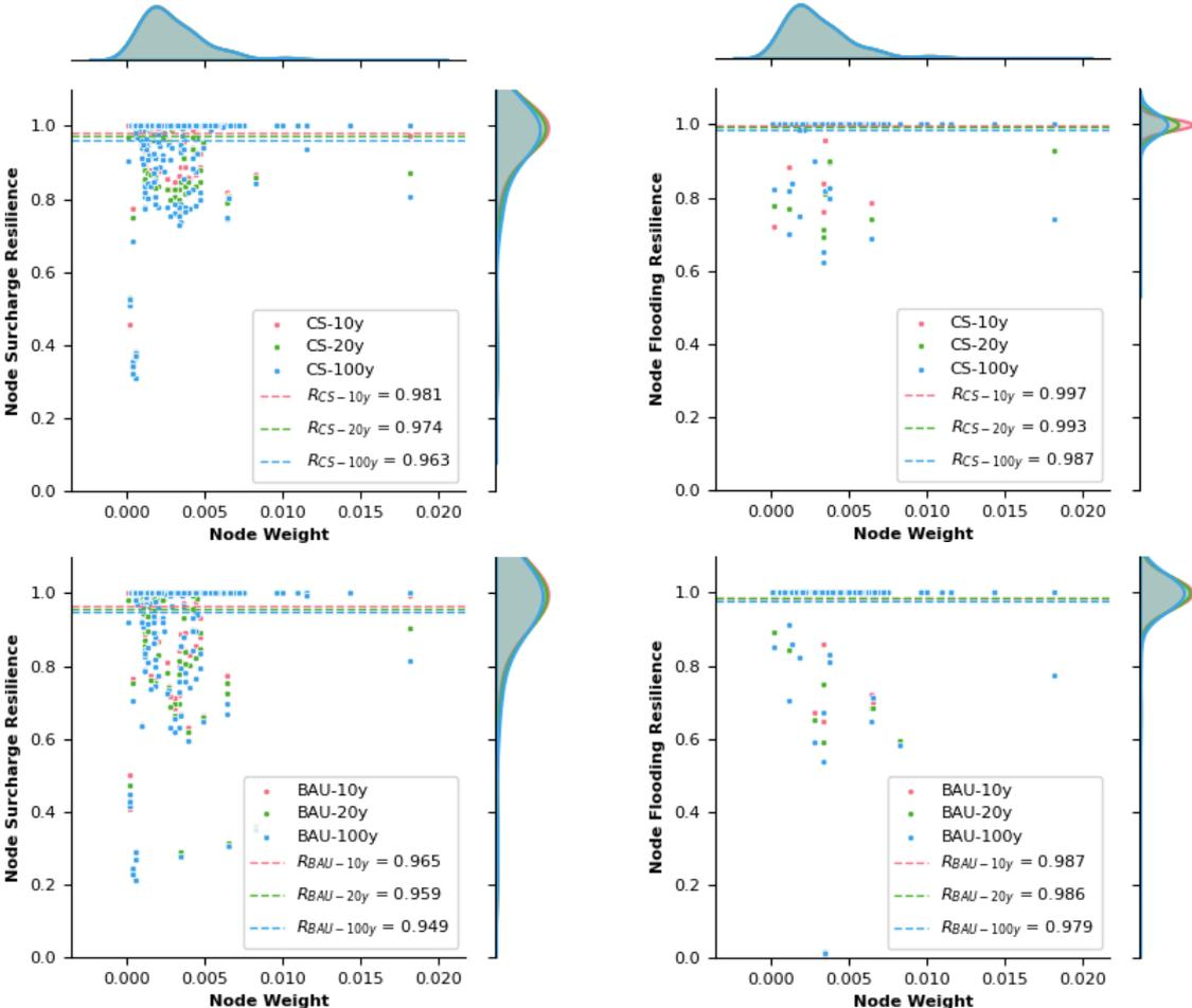
**Figure 6-23.** Plots of node weights vs. node surcharge resilience (left) and node weights vs. node flooding resilience (right) for the CS (top), BAU (middle), and FS (bottom) in the Historic Downtown catchment
