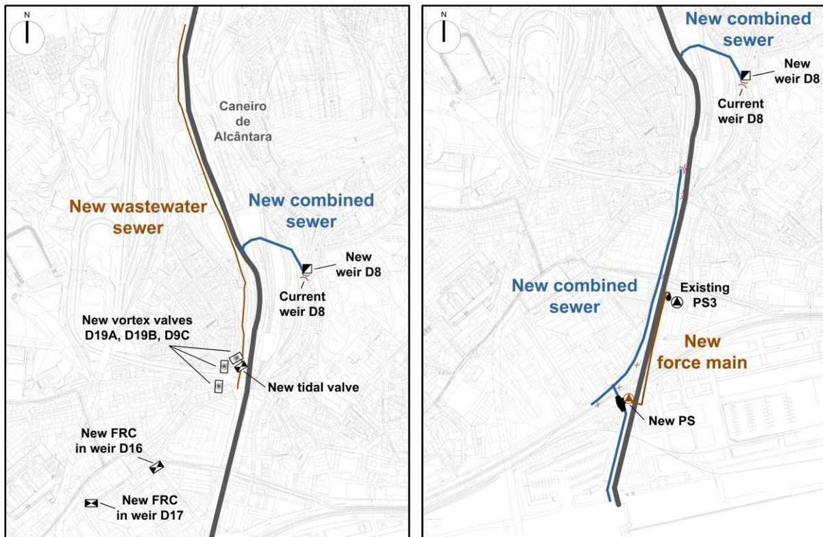
**Figure 6-15.** Schematic representation of main interventions regarding AS1 (left) and AS2 (right) (adapted from HIDRA, 2019). FRC stands for Flow Regulation Chamber
