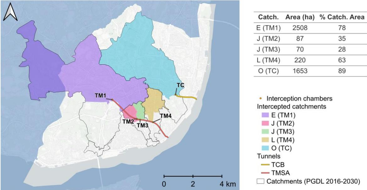
Figure 6-14. Tunnels: associated drainage catchments and intersection locations (HIDRA, 2018)
