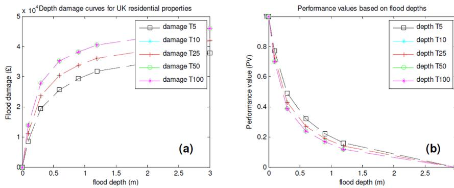
**Figure 3-16.** Example of depth-damage curves (a) and derived depth-performance curves (b) (Mugume et al., 2014)
