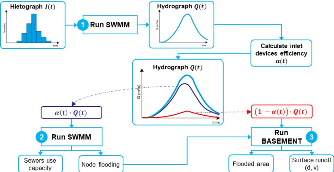
**Figure 6-1.** Loosely-coupling procedure for SWMM/BASEMENT modeling
