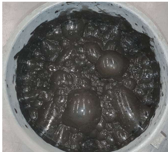
Figure 4 - H 2 gas formation in the preparation of mortars
