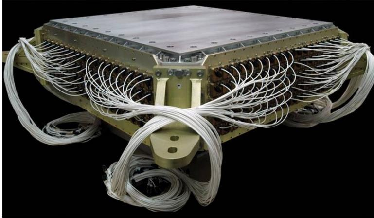
**Figure 4.6:** Photography of the Electromagnetic Calorimeter [48].
