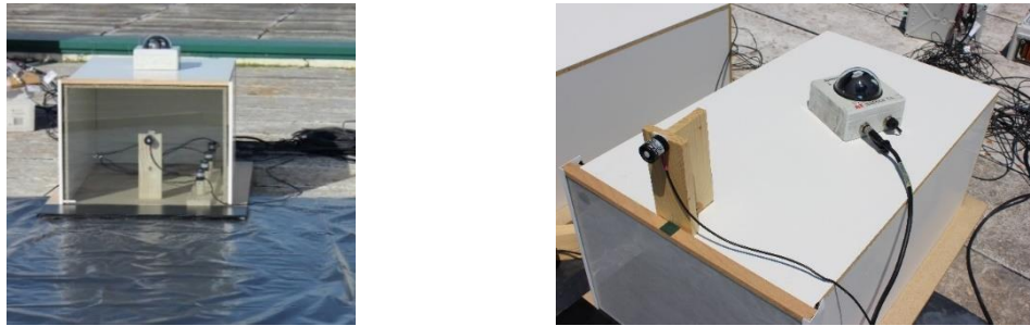
Figure 25. Small scale model (1:10) on the rooftop of DECivil building in IST, Portugal
