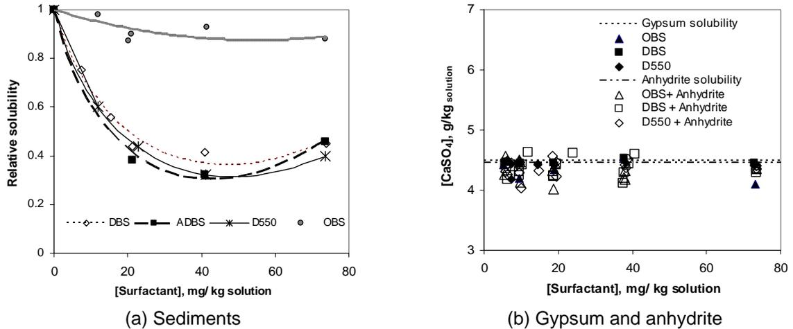
Figure 2 - Effect of the type and concentration of OBS, DBS, ADBS and D550 on the dissolution of calcium sulfate after 14 days of curing
