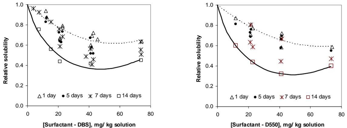
Figure 3 – Influence of the solid-liquid contact time on the dissolution of sediments S3 for several initial contents of two C<sub>12</sub>BS surfactants
