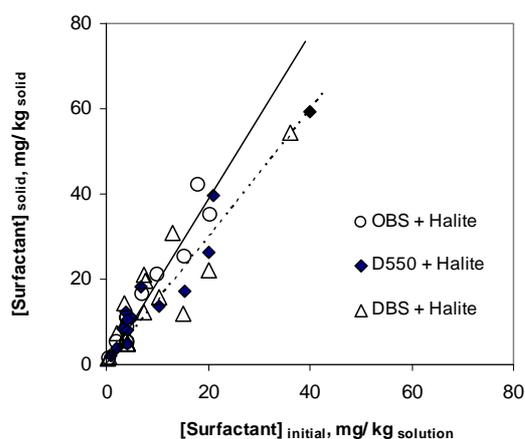
Figure 6 – Surfactants retention in halite crystals after 7 days of solid-liquid contact
