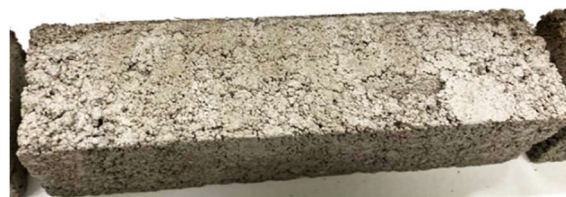
Figure 12 - Efflorescence in MIBA mortars
