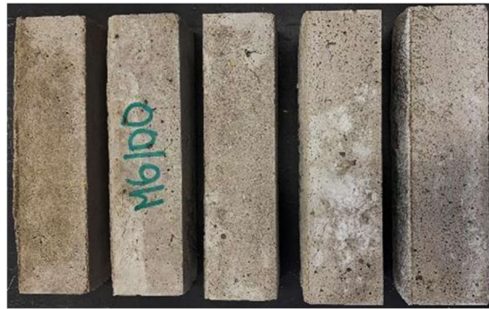
Figure 12 - Efflorescence in MIBA mortars
