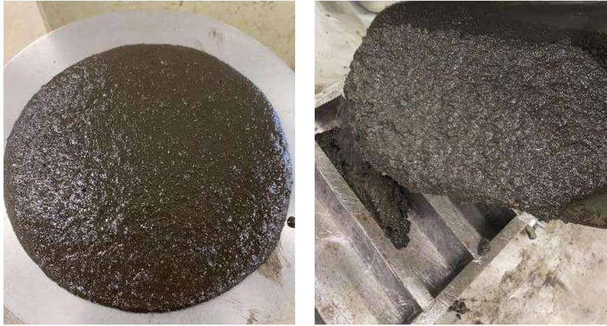
Figure 7 - Foaming MIBA in fresh state
