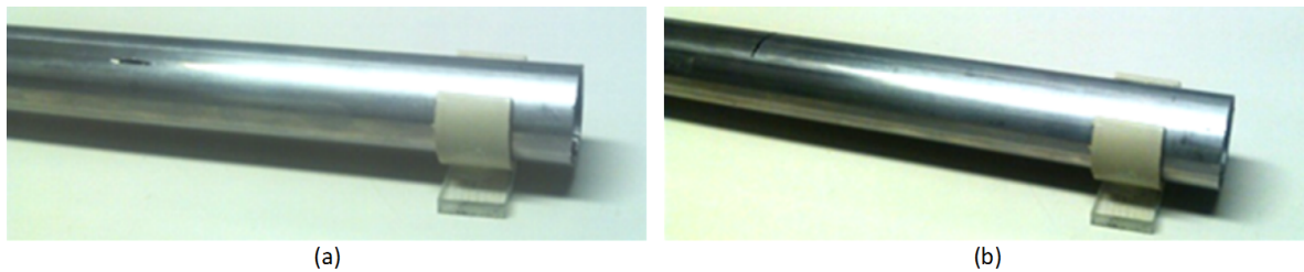
Figure 6.13: Photographs of the stainless steel tubes under test: (a) Sample tube with the longitudinal defect; (b) Sample tube with the transversal defect.
