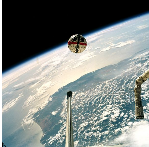
Figure 1.3: The Autonomous Extravehicular Activity Robotic Camera Sprint (AERCam Sprint), a prototype free-flying television camera, as seen from the cargo bay of the Space Shuttle Colombia during mission STS-87. AERCam was teleoperated from the shuttle during the experiment. [Credit: NASA, 1997]
