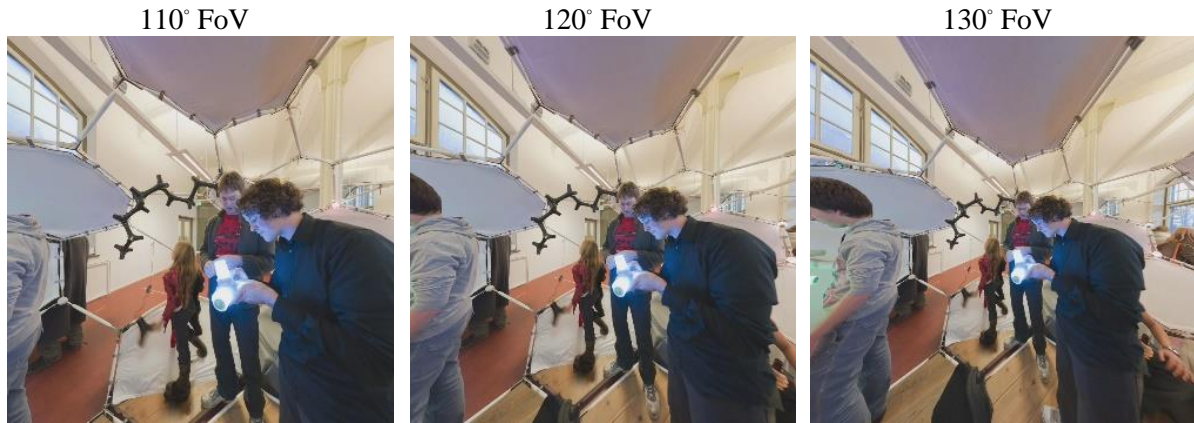
Figure 1.5. Example of viewports obtained with the rectilinear projection and varying FoV.
