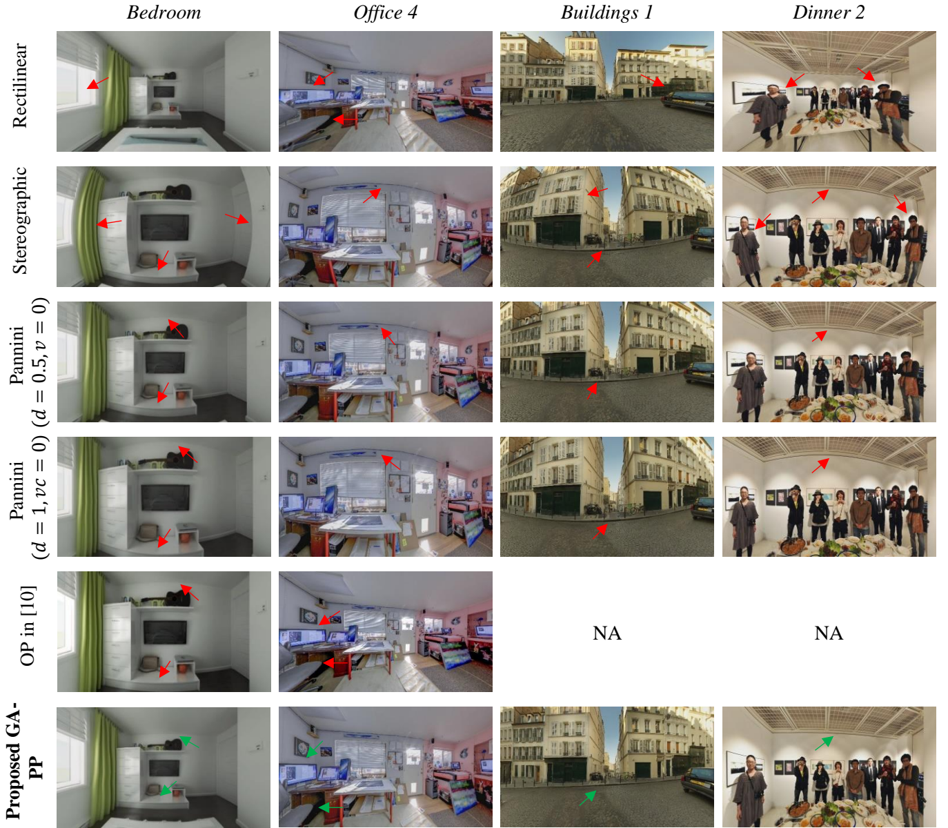
Figure 6.4. Example of viewports rendered with different projections and using a horizontal FoV of 150^\circ . NA corresponds to Not Available. The red and green arrows indicate, respectively, objects/regions with high and low geometric distortions.
