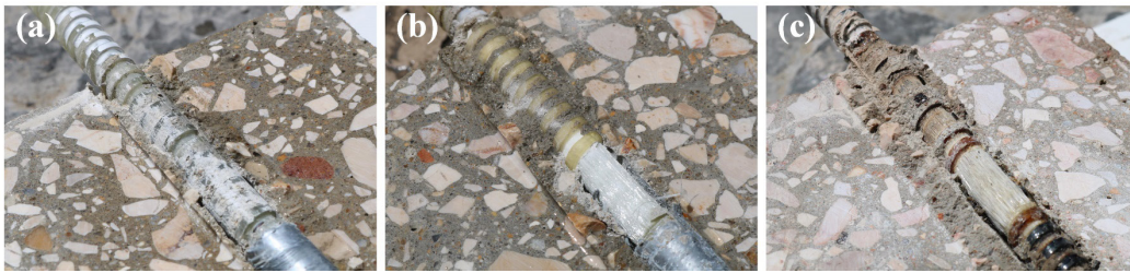
Figure 4.11. Specimens RBP-S representative of pull-out tests at: (a) 20 °C, (b) 100 °C-220 °C; (c) 300 °C.
