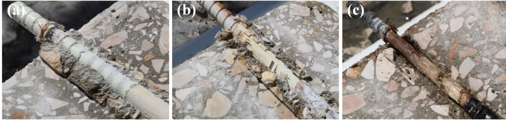
Figure 4.10. Specimens RB-D12 and RB-D8 representative of pull-out tests at: (a) 20 °C-140 °C, (b) 170 °C-250 °C; (c) 300 °C.
