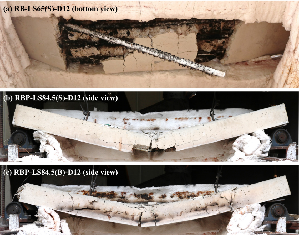
Figure 6.34. View of slabs with spliced reinforcement after failure: (a) RB-LS65(S)-D12, (b) RBP-LS84.5(S)-D12 and (c) RBP-LS84.5(B)-D12.
