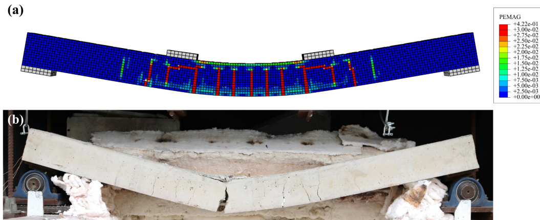
Figure 7.8. Side view of (a) numerical (including the plastic strain magnitude field – PEMAG [-]) and (b) experimental failure modes of slab SC-LS65(S)-D10-II under thermomechanical loading.
