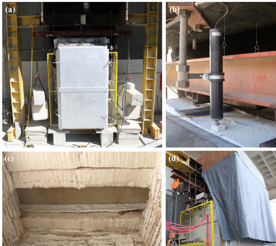
Figure 6.12. Fire resistance tests setup: (a) general view during loading stage; (b) displacement transducers installed at midspan; (c) bottom view of the slab; (d) general view during the tests.
