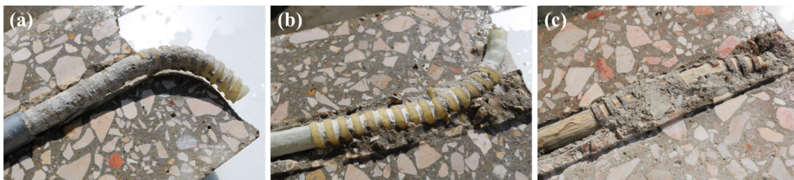
Figure 4.16. Surface of RBP-B bars after being tested at: (a) 20 °C, (b) 100 °C-220 °C; (c) 300 °C.
