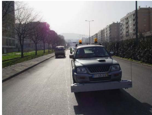
Figure 6.5 – Picture of the High Speed Profilometer (HSP) system.
