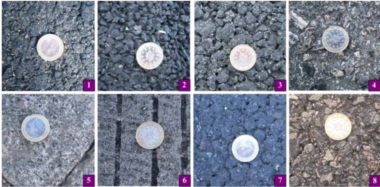
Figure 6.6 – Pavement types tested in this study (database db1). 1- porous asphalt1 (PA1) (new), 2- gap graded asphalt rubber (GGAR), 3- rough thin layers (RTL), 4- dense asphalt (DA) (old), 5- cubic paving stones (PCS), 6- cement concrete (CC), 7- asphalt recycled rubber (ARR-BMB), 8 - porous asphalt 2 (PA2).
