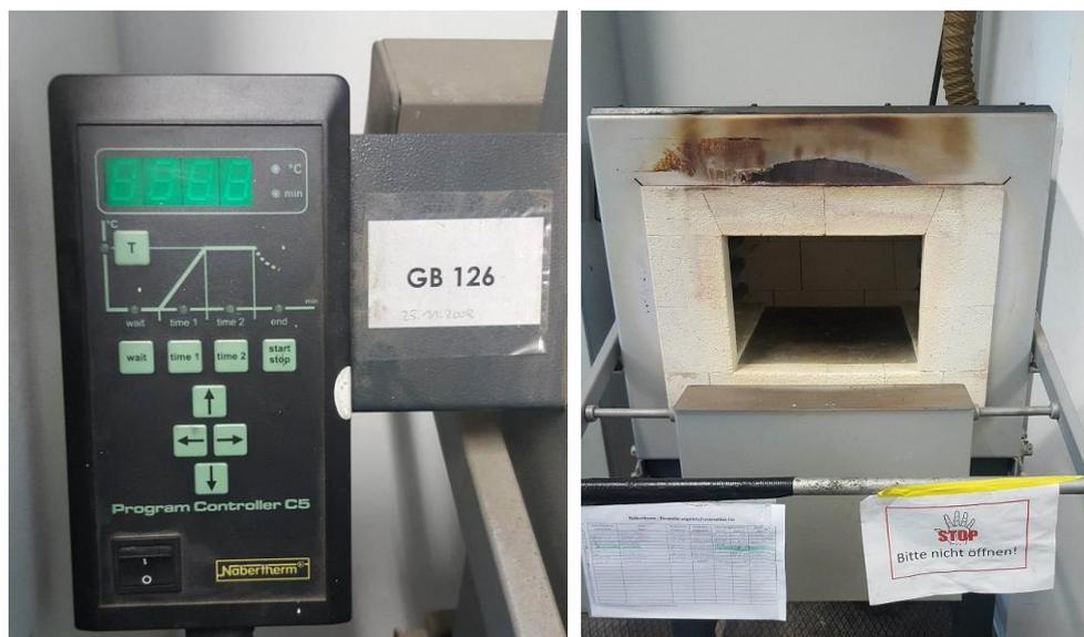
Figure 3.6: Temperature program controller (left) and muffle furnace (right).
