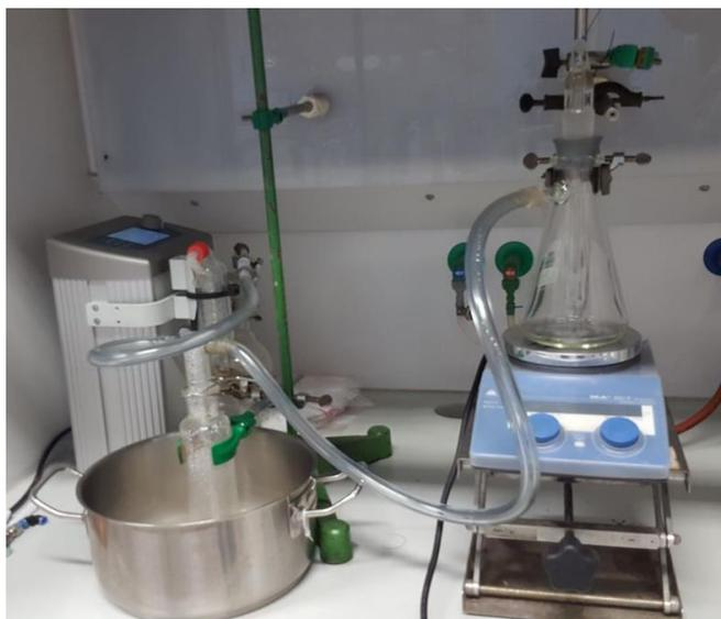
Figure 3.7: Evaporation device.
