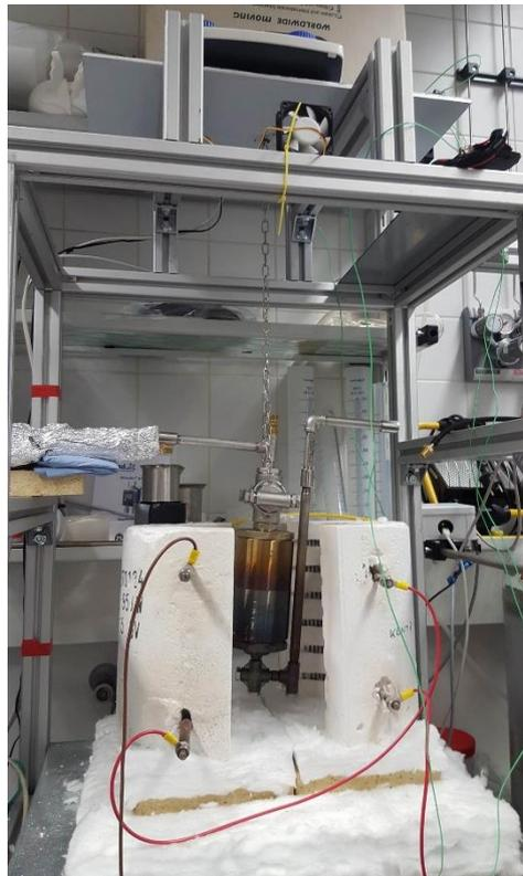
Figure 3.3: Reactor used in the TGA apparatus.
