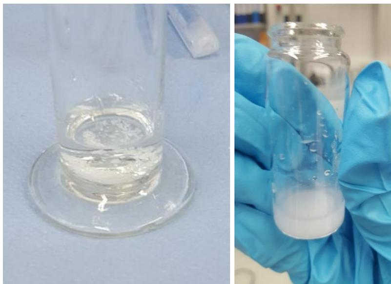
Figure 5.6: Rehydration of boron oxide produced in the muffle furnace (left) and in the evaporation device (right) using 7 mL of water.
