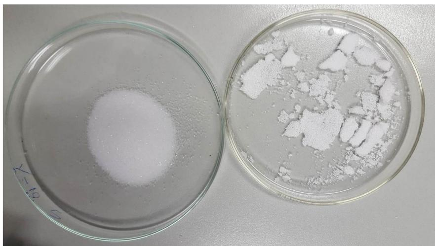
Figure 4.18: Difference between sheer boric acid(left) and generated boron oxide (right).
