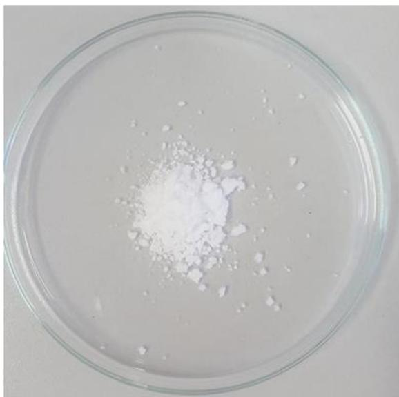
Figure 4.19: Boron oxide after dehydration with generated boric acid.
