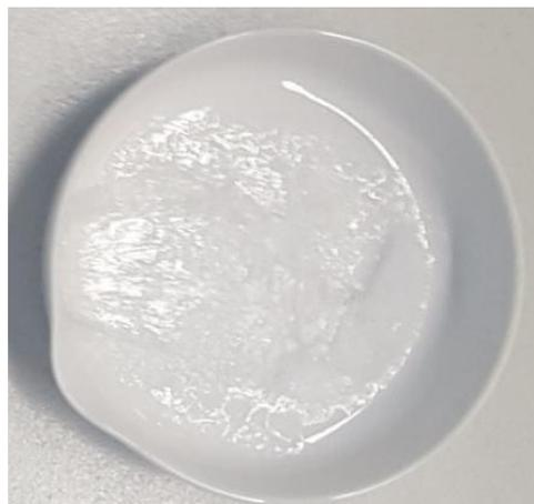
Figure 4.14: Dehydration for 10 min at 350°C.
