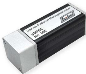
**Figure 4.5:**  $\mu$ Spec500 detector. [7]
